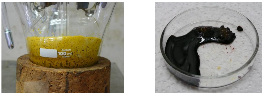
Fig. 2 Crystalline (C_4mim)_2CuCl_3 at ambient temperatures under inert atmosphere (l) and after being exposed to air for several minutes (r).
