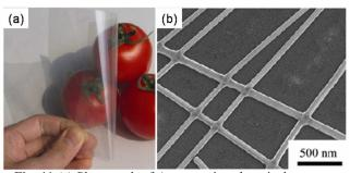
**Fig. 11** (a) Photograph of Ag nanowires deposited on a transparent PET substrate and (b) FE-SEM images of Ag NWs on a PET substrate after mechanical processing. (Reproduced with permission from ref. 136)
