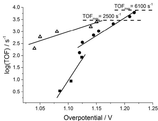
**Figure 6.** The TOF increase vs overpotential accompanying the addition of acid. The experimental points for: **PdTFcP** and TFA – triangles, **CuTFcP** and TFA – dots, **CuTFcP** and TEAHCl – squares. Solid line is showing the changes trend and dashed line is showing the maximum TOF at which catalytic current stops to increase with addition of acids.
