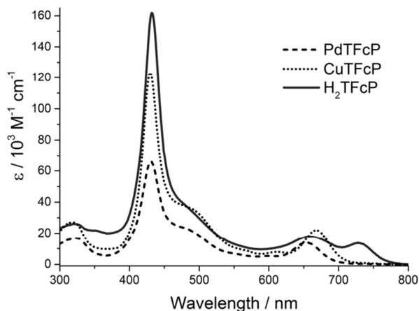
**Figure 3.** Room temperature UV-Visible absorption spectra for **H<sub>2</sub>TFcP**, **CuTFcP** and **PdTFcP** in THF.
