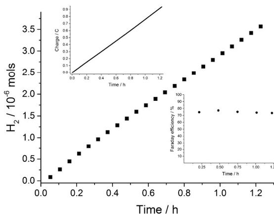
**Figure 8.** Electrocatalytic hydrogen production vs time, charge vs time (left top insert) and Faradaic efficiency vs time (right bottom insert) by applying -1.5 V vs SCE to a glassy carbon electrode in 0.2 M TBABF<sub>4</sub> solution of DMF containing 50 mM TEAHCl and 0.1 mM **CuTFcP**.
