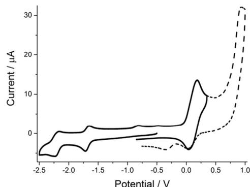
**Figure 2.** Cyclic voltammogram recorded for **PdTFcP** in DMF containing 0.2 M TBATFB vs.  $\text{Fe}(\text{Cp})_2^+/\text{Fe}(\text{Cp})_2$ . The dashed line shows the additional irreversible oxidation peak when the potential window was increased.
