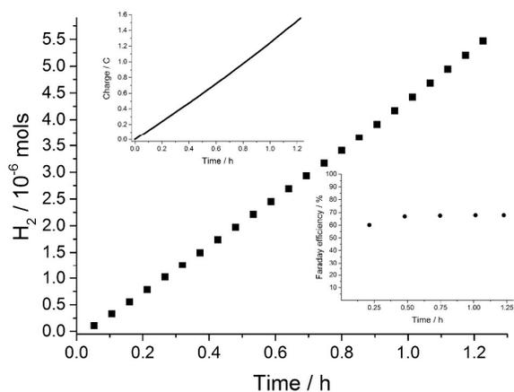
**Figure 7.** Electrocatalytic hydrogen production vs time, charge vs time (left top insert) and Faradaic efficiency vs time (right bottom insert) by applying -1.5 V vs SCE to a glassy carbon electrode in 0.2 M TBABF<sub>4</sub> solution of DMF containing 50 mM TFA and 0.1 mM **CuTFcP**.
