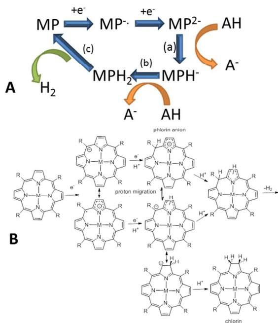
**Scheme 1.** (A) Simplified diagram showing the electrocatalytic formation of hydrogen from a metalloporphyrin (MP). (B) Potential products from the series of reduction and protonation processes. Note: at high concentration of acid the first protonation could take place at the porphyrin monoanion.
