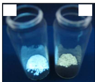
Figure 7. Photo of 1%Dy: Y_2WO_6 before heat treatment (a) and after heat treatment (b) when placed under a UV lamp with a 254 nm excitation wavelength.
