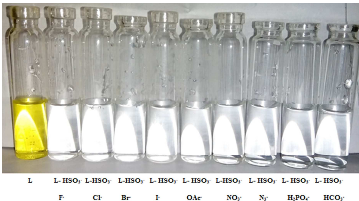
Fig. 12 The colour changes of L and its complexation with \text{HSO}_3^- in the presence of various anions in MeOH-H 2 O (2:1, v/v) at room temperature. Conditions: L , 10 \mu\text{M} ; \text{HSO}_3^- , 10 equiv.; other anions, 10 equiv.
