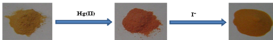
Fig. 11: Photographs of surface modified silica gel SiR-1 , ( SiR-1 )-Hg(II), ( SiR-1 )-Hg(II) + KI (from left to right).
