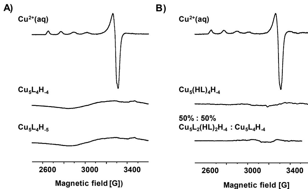
**Figure 4.** Representative EPR spectra registered for: A) Cu(II) and Ac-KLH-NHOH at the 1:1 metal:ligand ratio,  $C_{\text{Cu(II)}} = 0.80 \times 10^{-3} \text{M}$ ; B) Cu(II) and [AH]-NHOH as a function of pH at the 1:1 metal:ligand ratio,  $C_{\text{Cu(II)}} = 0.80 \times 10^{-3} \text{M}$ .
