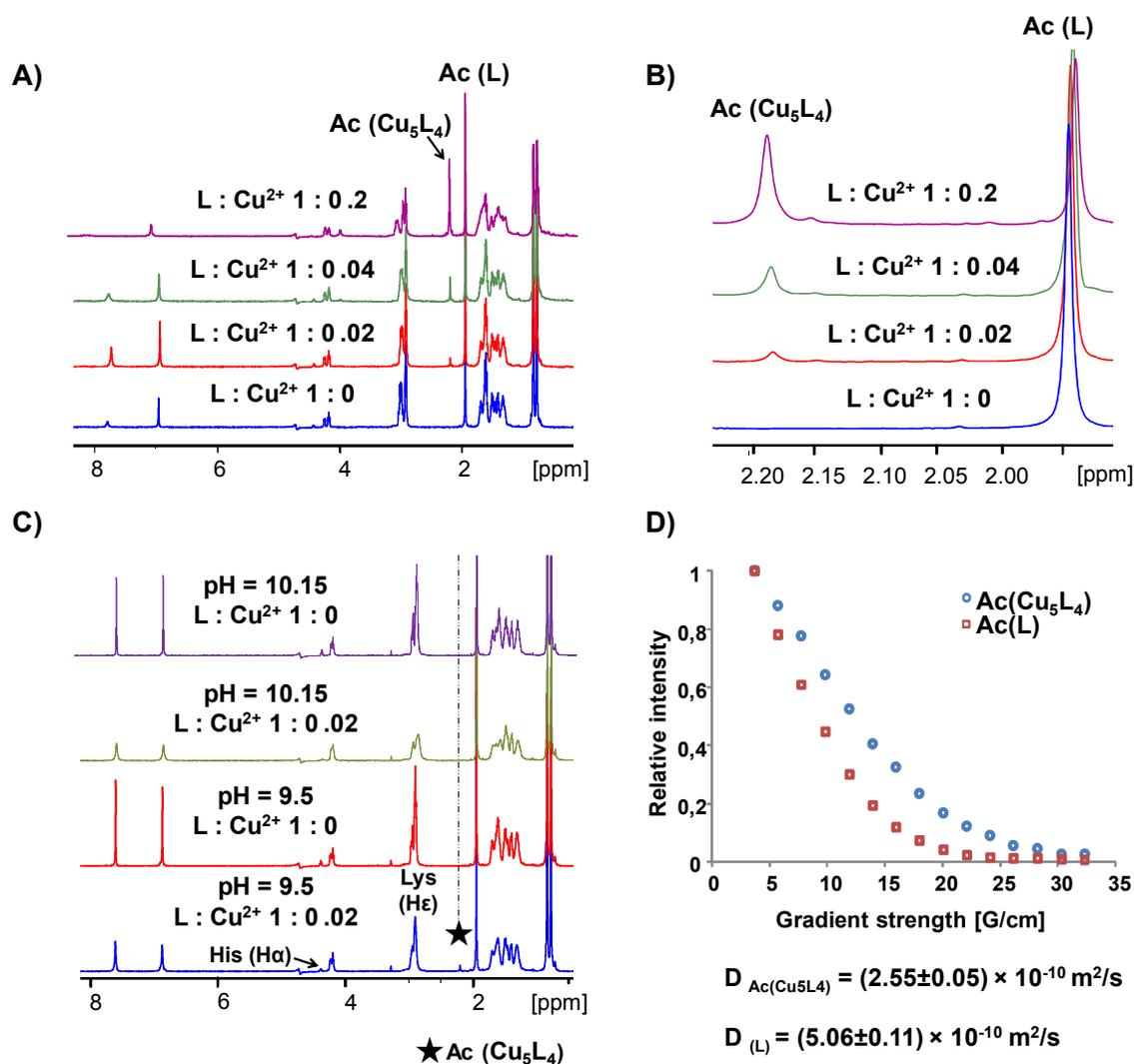
**Figure 6.** The  $^1\text{H}$  NMR spectra of Ac-KLH-NHOH in the presence of  $\text{Cu}^{2+}$  ions. A) Spectra measured at pH 6.8 at various metal:ligand ratios; B) enlarged parts of spectra from A showing the appearance of a signal corresponding to the Ac(Cu<sub>5</sub>L<sub>4</sub>) metallacrown acetyl group (acetyl group protects the N-terminal amino group of the peptide) besides the peak corresponding to the free peptide acetyl group; C) Comparison of the spectra of the complex
