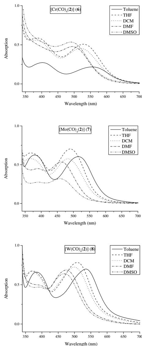
**Figure 11:** Absorption spectra of the bipyridine-based complexes **6-8** measured in the solvent range from nonpolar toluene to highly polar DMSO at  $T = 298$  K from  $1.25 \cdot 10^{-4}$  M solutions.
