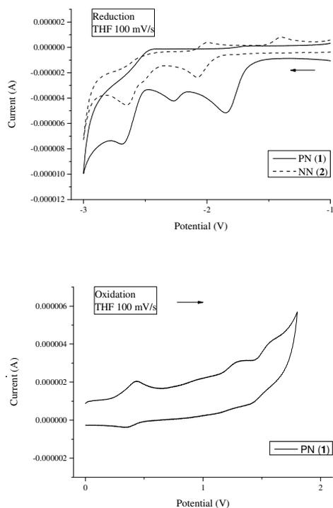
**Figure 12** Electrochemical spectra of ligand **1** and **2** determined by CV on a glassy carbon working electrode in 0.1 M  $n\text{Bu}_4\text{NPF}_6$  and  $5 \cdot 10^{-3}$  M THF solutions at  $T = 298$  K.
