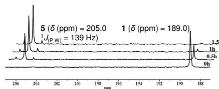
**Figure 5:** Time-dependent  $^{31}\text{P}\{^1\text{H}\}$  NMR spectra for the ligand exchange of the bipyridine derivative **2** by the P,N hybrid ligand **1** under formation of complex **5** in toluene at  $T = 120^\circ\text{C}$ .
