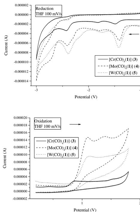
**Figure 13** Electrochemical spectra of phosphinine-based coordination compounds **3-5** determined by CV on a glassy carbon working electrode in 0.1 M  $n\text{Bu}_4\text{NPF}_6$  and  $5 \cdot 10^{-3}$  M THF solutions at  $T = 298$  K.
