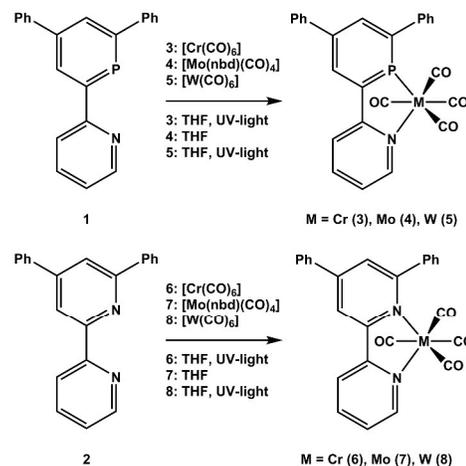
**Scheme 1:** Synthesis of tetracarbonyl complexes **3-8** containing **1** and **2**.
