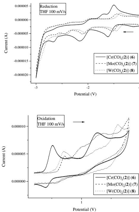
**Figure 14** Electrochemical spectra of bipyridine-based coordination compounds **6-8** determined by CV on a glassy carbon working electrode in 0.1 M  $n\text{Bu}_4\text{NPF}_6$  and  $5 \cdot 10^{-3}$  M THF solutions at  $T = 298$  K.
