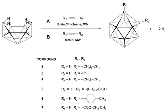
**Figure 2.** Scheme of the reaction for the preparation of *o*-carborane derivatives using microwave (MW) heating; Route A: Using ionic liquids; route B: Using acetonitrile both as the Lewis base and the solvent.
