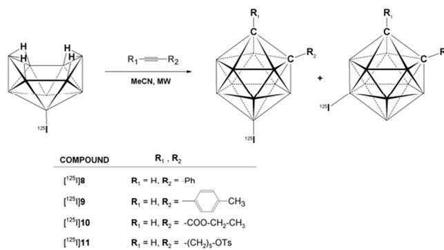
**Figure 3.** Scheme of the reaction for the preparation of <sup>125</sup>I-labelled *o*-carborane derivatives using microwave (MW) heating and acetonitrile as Lewis base and solvent in a one-step, one-pot reaction. The same strategy was used for the preparation of <sup>131</sup>I-labelled analogues.
