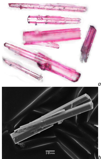
Fig.1 Photo of crystals of the title compound (a) and SEM image, showing the prismatic morphology of the studied crystal (b)
