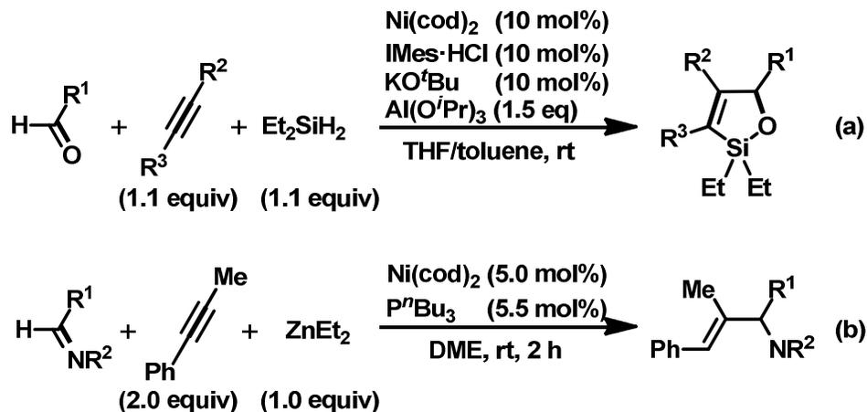
**Scheme 13.** (a) Nickel(0)-catalyzed cyclocondensation reaction of aldehydes, alkynes, and  $\text{Et}_2\text{SiH}_2$  and (b) nickel(0)-catalyzed reductive coupling of imines, alkynes, and  $\text{ZnEt}_2$ .<sup>15,16</sup>
