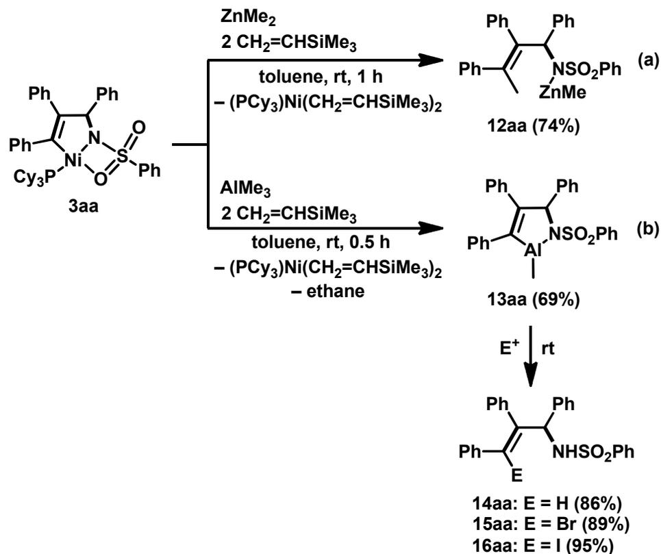
**Scheme 10.** Reaction of five-membered aza-nickelacycle **3aa** with methylmetal reagents. Yields of isolated products are given. Reaction conditions: for **14aa**, MeOH/toluene, instance; for **15aa**, NBS (2 equiv) in  $\text{CH}_3\text{CN}$ , 0.5 h; for **16aa**,  $\text{I}_2$  (excess) in  $\text{CH}_3\text{CN}$ , 2 h, then HCl.
