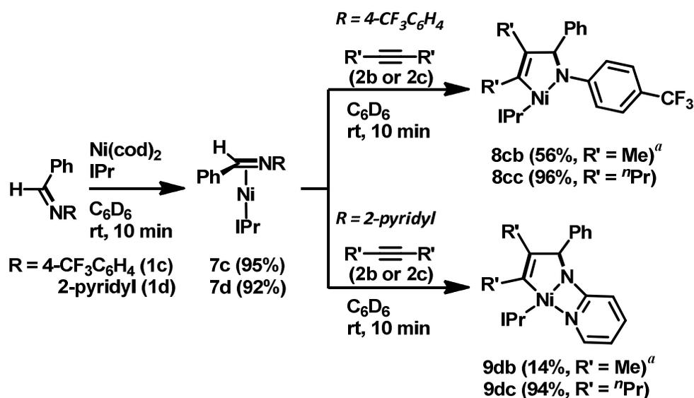
**Scheme 5.** The stoichiometric reactions using *N*-aryl imines and alkynes with Ni(0)/IPr. Yields were determined by  $^1\text{H}$  NMR spectroscopy. *a)* The reaction was carried out in toluene. Isolated yields after recrystallization are shown.
