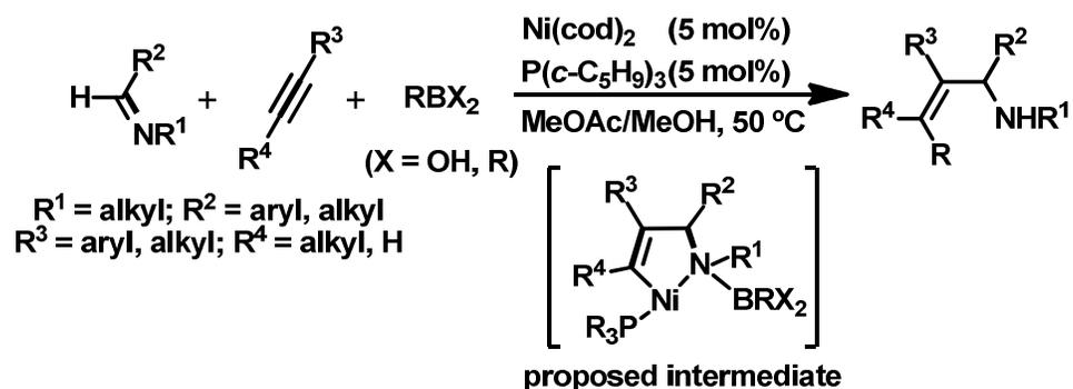
**Scheme 11.** Nickel(0)-catalyzed three-component coupling reaction of alkynes, imines, and organoboron reagents.<sup>13</sup>
