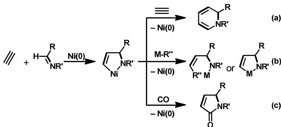
**Scheme 1.** Formation of five-membered aza-nickelacycles generated via oxidative cyclization of an imine and an alkyne, and their key role in the nickel-catalyzed transformation reactions leading to nitrogen-containing products.
