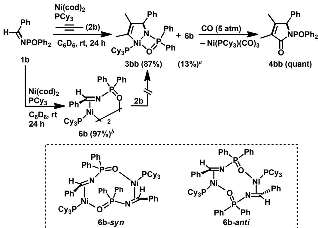
**Scheme 4.** Formation of five-membered aza-nickelacycle **3bb** and its reactivity with carbon monoxide.
