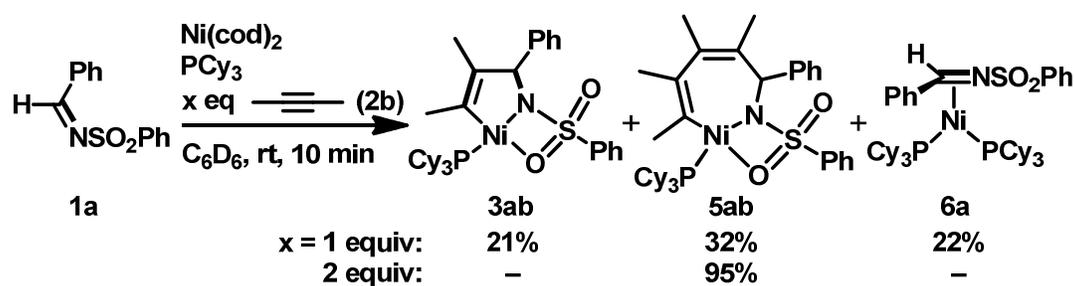
**Scheme 3.** Reaction of **1a** with **2b** (1 or 2 equiv) in the presence of Ni(0)/PCy<sub>3</sub>. Yields, determined by <sup>1</sup>H NMR spectroscopy, are given.
