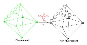
Scheme 1 Fluorescent MOF 1 based sensor for highly selective nitro explosive detection in aqueous phase.
