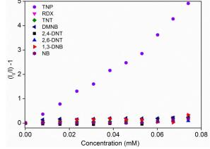
Fig. 2 Stern-Volmer plots for nitro analytes added to 1' in water.
