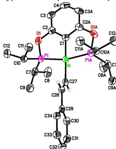
**Fig. 2** ORTEP drawing of (*E*)-[2,6-(<sup>i</sup>Pr<sub>2</sub>PO)<sub>2</sub>C<sub>6</sub>H<sub>3</sub>]NiCH=CHPh (**6a**) at the 50 % probability level. Selected bond lengths (Å) and angles (°): Ni–C(1) 1.903(4), Ni–C(27) 1.924(4), Ni–P(1) and Ni–P(1A) 2.1270(8), C(27)–C(28) 1.276(6), C(28)–C(29) 1.494(5), P(1)–Ni–P(1A) 164.40(5), C(1)–Ni–C(27) 179.55(18).
