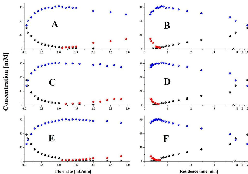
**Fig. 3** Transesterification of neopentylglycol in a biphasic (50/50 % v/v) system of buffer/ethyl acetate by MsAcT covalently immobilised on amino modified monolith (A, B), adsorbed by His-tag on: Ni-modified monolith (C, D) and on Co modified monolith (E, F). Conditions: 0.05 M phosphate buffer pH 7.5; 96 mM neopentylglycol in ethyl acetate; room temperature. (red) substrate, (black) diester, (blue) monoester.
