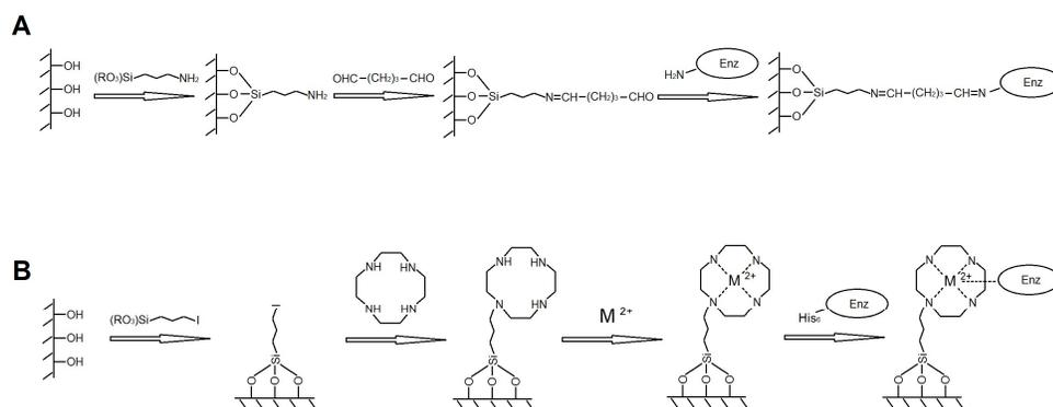
**Scheme 2** Functionalisation of silica carriers and immobilisation of MsACT by covalent bonding (A) and specific His-tag-mediated adsorption on Ni/Co sites (B).
