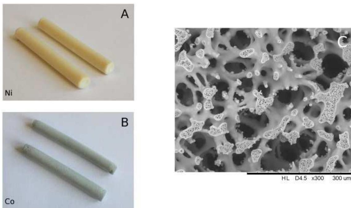
**Fig. 2** Silica monoliths with Ni (A), and Co (B). SEM image of monolith structure (C).
