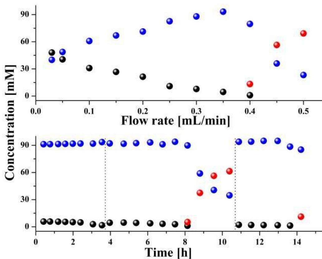
**Fig. 5** Transesterification of neopentylglycol in absence of buffer by MsAcT adsorbed by His-tag on Ni-modified monolith (A) and process stability (flow rate 0.1 mL/min) (B). Conditions: 96 mM neopentylglycol in ethyl acetate; room temperature. (red) substrate, (black) diester, (blue) monoester. Vertical lines show the interruptions in measurements, the immobilised enzyme was washed and stored in buffer.
