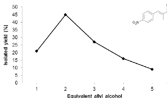
Figure 2 Effect of allyl alcohol excess on the reaction of 4-nitrobenzaldehyde with allyl alcohol. (Reaction conditions: 0.5 mmol aldehyde, 1 mL toluene, 5 mol% Pd (source: 5 % \text{Pd}/\text{Al}_2\text{O}_3 ), 0.5 mmol \text{K}_2\text{CO}_3 , 100^\circ\text{C} , 24 h.)
