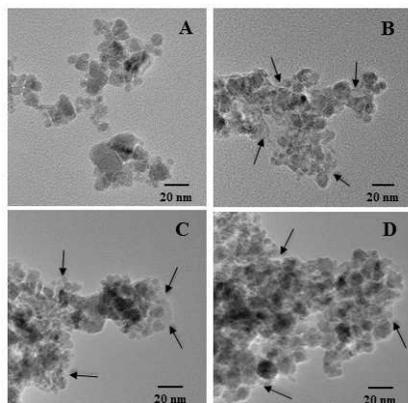
**Fig. 2** Typical TEM images of (A) free MNPs, (B) Mb-MNPs<sub>1mg</sub>, (C) Mb-MNPs<sub>5mg</sub>, and (D) Mb-MNPs<sub>10mg</sub> conjugates. The Mb films around MNPs in each conjugate are indicated by arrow heads.
