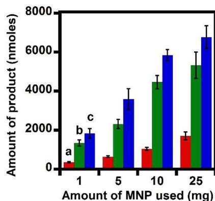
**Fig. 4** ABTS oxidation product yields catalyzed by (a) free MNPs, (b) free Mb, and (c) Mb-MNPs<sub>1mg</sub> conjugates. The corresponding comparative data for samples of Mb-MNPs<sub>5mg</sub> and Mb-MNPs<sub>10mg</sub> along with the respective free MNPs and free Mb controls are also shown as labeled in the x-axis. ABTS oxidation was carried out in PBS solution in the presence of hydrogen peroxide (1 mM) at 25 °C, pH 7.4.
