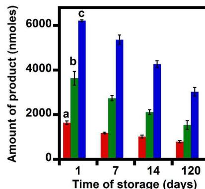
Fig. 7 Storage stability of the Mb-MNP conjugates prepared using (a) 1, (b) 5, and (c) 10 mg of MNPs. Oxidation of 10 mM ABTS in the presence of 1 mM H<sub>2</sub>O<sub>2</sub> in PBS solution (pH 7.4), 25 °C was tested on the initial day of the experiment and after 7, 14, and 120 days of storage at 4 °C.
