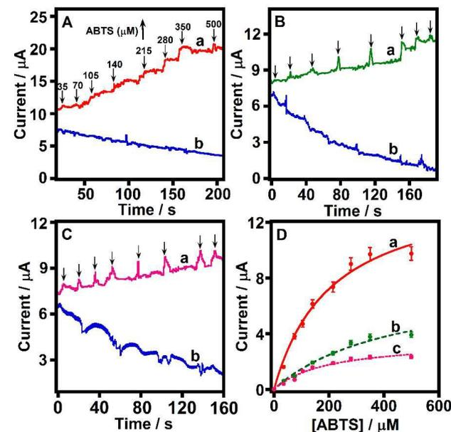
Fig. 8 Amperometric data (i-t curves) for ABTS oxidation by (A) (a) HPG/Mb-MNPs<sub>10mg</sub> and (b) only HPG/MNPs<sub>10mg</sub> (no Mb control); (B) (a) HPG/Mb-MNPs<sub>5mg</sub> and (b) only HPG/MNPs<sub>5mg</sub> (no Mb control); and (C) (a) HPG/Mb-MNPs<sub>1mg</sub> and (b) only HPG/MNPs<sub>1mg</sub> (no Mb control) in PBS, pH 7.4 under saturated atmospheric air conditions at an applied potential of  $-0.5$  V vs. Ag/AgCl, 150 rpm electrode rotation rate, 25 °C. (D) Electrochemical
