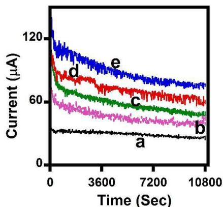
**Fig. 10** Electrocatalytic stability (i-t curve) of (a) MNPs, (b) Mb, (c) HPG/Mb-MNPs<sub>1mg</sub>, (d) HPG/Mb-MNPs<sub>5mg</sub>, and (e) HPG/Mb-MNPs<sub>10mg</sub> in buffer pH 7.4 PBS under saturated atmospheric air conditions at an applied potential of  $-0.5$  V vs. Ag/AgCl, 150 rpm rotation rate, 25 °C.
