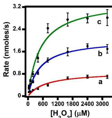
**Fig. 5** The Michaelis-Menten kinetics of (a) MNPs, (b) Mb in solution, and (c) Mb-MNPs<sub>1mg</sub> toward ABTS oxidation under various concentrations of  $\text{H}_2\text{O}_2$ .
