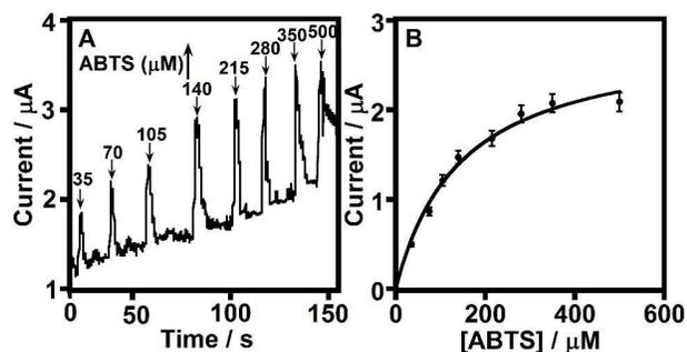
**Fig. 9** (A) Amperometric data (i-t curve) for ABTS oxidation by HPG/Mb electrodes without MNP conjugation in PBS buffer (pH 7.4) under saturated atmospheric air conditions at an applied potential of  $-0.5$  V vs. Ag/AgCl, 150 rpm rotation rate, 25 °C. (B) Electrochemical Michaelis-Menten kinetics of ABTS electrolysis by HPG/Mb electrodes.
