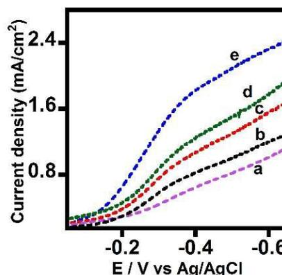
**Fig. 11** Representative steady-state catalytic reduction voltammograms of *t*-BuOOH (5 mM), oxygen-free PBS, 25 °C catalyzed by: (a) free MNPs, (b) free Mb, (c) Mb-MNPs<sub>1mg</sub>, (d) Mb-MNPs<sub>5mg</sub>, and (e) Mb-MNPs<sub>10mg</sub> conjugates adsorbed on HPG electrodes, scan rate 0.3 Vs<sup>-1</sup>, 1000 rpm electrode rotation rate.
