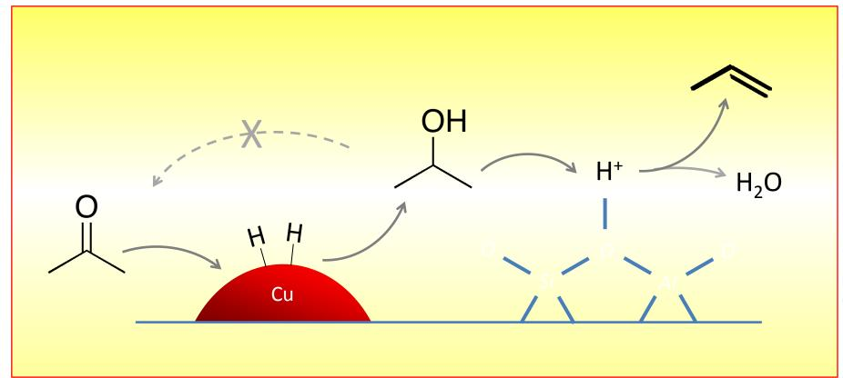
Hydrogenation of a ketone primarily takes place on the metal surface resulting in a corresponding alcohol that can be dehydrated to olefin over the acid function. A rapid dehydration synergistically prevent reversible dehydrogenation of alcohol while excessive olefin hydrogenation can be limited over selected metal.
