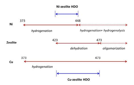
For  $Cu/SiO_2$  - zeolite system, no hydrogenolysis can be promoted up to 575 K (Figure 3). However, the reaction over acid site is limited at 473 K to avoid the drastic oligomerization. Accordingly, the window for hydrodeoxygenation over  $Cu/SiO_2$  - zeolite system is widely opened (423 – 473 K), as illustrated above.
