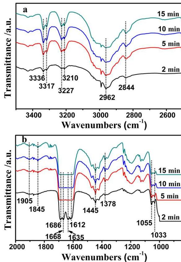
Fig. 5. *In situ* DRIR spectra of MN on (Pd-CuCl<sub>2</sub>)/ $\gamma$ -Al<sub>2</sub>O<sub>3</sub> catalyst at 120 °C: (a) range from 3500 to 2500 cm<sup>-1</sup>; (b) range from 2000 to 1000 cm<sup>-1</sup>.
