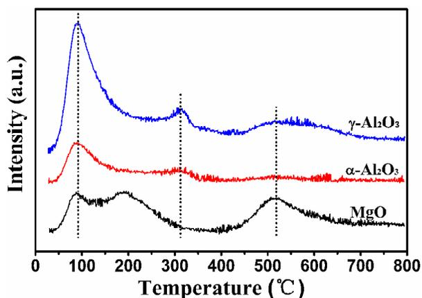
**Fig. 2.** NH<sub>3</sub>-TPD profiles of Pd-CuCl<sub>2</sub> catalysts with different supports.
