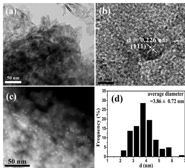
**Fig. 1.** (a) TEM, (b) HRTEM, (c) STEM images and (d) size distributions of Pd nanoparticles of (Pd-CuCl<sub>2</sub>)/ $\gamma$ -Al<sub>2</sub>O<sub>3</sub> catalyst.
