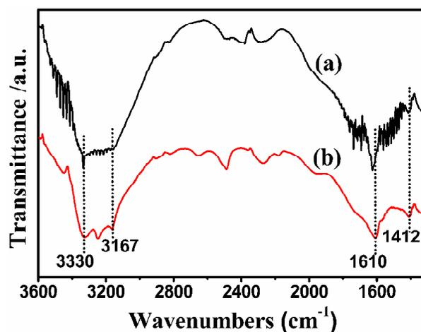
**Fig. 3.** NH<sub>3</sub>-FTIR spectra of (Pd-CuCl<sub>2</sub>)/ $\gamma$ -Al<sub>2</sub>O<sub>3</sub> catalyst: (a) exposure to NH<sub>3</sub>, (b) swept by N<sub>2</sub>.
