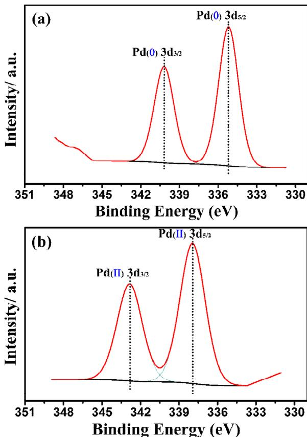
Fig. 4. Pd 3d XPS spectra of (a) fresh and (b) engaged (Pd-CuCl<sub>2</sub>)/ $\gamma$ -Al<sub>2</sub>O<sub>3</sub> catalysts.
