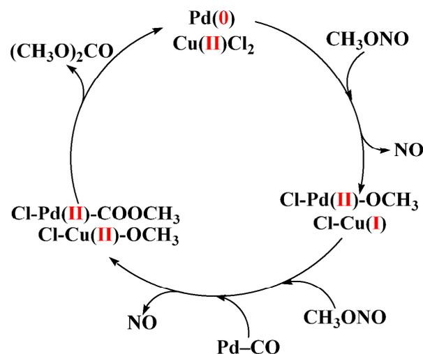
Fig. 7. The proposed catalytic mechanism of DMC formation on (Pd-CuCl<sub>2</sub>)/ $\gamma$ -Al<sub>2</sub>O<sub>3</sub> catalyst.
