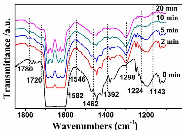
Fig. 6. *In situ* DRIR spectra of the reaction between CO and MN on (Pd-CuCl<sub>2</sub>)/ $\gamma$ -Al<sub>2</sub>O<sub>3</sub> catalyst at 120 °C, range from 1850 to 1100 cm<sup>-1</sup>.
