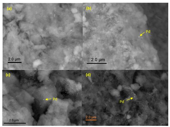
Fig. 3. SEM images of (a) calcined-reduced  $Pd/Al_2O_3$ ; (b) used  $Pd/Al_2O_3$  from dry-VAM experiment; (c) used  $Pd/Al_2O_3$  from wet-VAM experiment; (d) used  $Pd/Al_2O_3$  from wet-dust-VAM experiment
