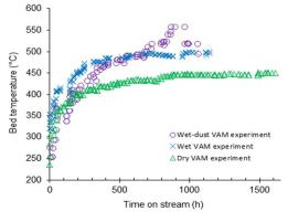
Fig. 1. Catalyst bed temperature required for 90 % CH<sub>4</sub> conversion over 1.0 Pd/Al<sub>2</sub>O<sub>3</sub> catalyst. Feed = 0.7 % CH<sub>4</sub>, 1 % CO<sub>2</sub>, 3-4 % H<sub>2</sub>O (for wet feeds) balance air. GHSV = 100000  $h^{-1}$ .  $\Delta$  = dry VAM experiment;  $\times$  = wet VAM experiment and  $\circ$ = wet-dust VAM experiment.
