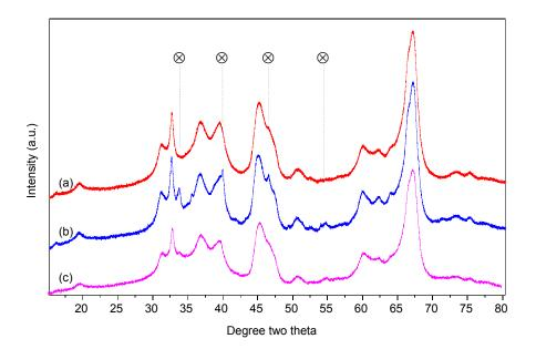
Fig. 7. XRD pattern of aged catalysts (a) Pd/Al<sub>2</sub>O<sub>3</sub>-I catalyst (aged 18 h in wet-feed at 780 °C); (b) Pd/Al<sub>2</sub>O<sub>3</sub>-II catalyst (aged 18 h in wet-feed at 830 °C); (c) Pd/Al<sub>2</sub>O<sub>3</sub>-III catalyst (aged 18 h in wet-O<sub>2</sub> at 780 °C). Phase:  $\otimes$  = PdO.
