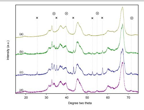
Fig. 2. XRD pattern of (a) calcined-reduced Pd/Al<sub>2</sub>O<sub>3</sub>, (b) used Pd/Al<sub>2</sub>O<sub>3</sub> of dry-VAM experiment, (c) used Pd/Al<sub>2</sub>O<sub>3</sub> wet-VAM experiment, (d) used Pd/Al<sub>2</sub>O<sub>3</sub> of wet-dust VAM experiment. Phase:  $\otimes$  = PdO and  $\times$  =  $\alpha$ -Al<sub>2</sub>O<sub>3</sub>
