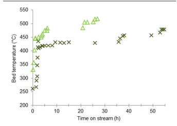
Fig. 6. Catalyst bed temperature required for 90 % CH $_4$  conversion over  $\Delta$  = Pd/Al $_2$ O $_3$ -III catalyst (aged 18 h in wet O $_2$  at 780 °C) and × = Pd/Al $_2$ O $_3$ -IV catalysts (aged 3 days in autoclave at 175 °C). Feed = 0.7 % CH $_4$ , 3.2 % H $_2$ O balance air. GHSV = 100 000 h $^{-1}$ .
