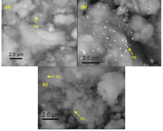
Fig. 8. SEM images of aged catalysts (a) Pd/Al<sub>2</sub>O<sub>3</sub>-I catalyst (aged 18 h in wet-feed at 780 °C); (b) Pd/Al<sub>2</sub>O<sub>3</sub>-II catalyst (aged 18 h in wet-feed at 830 °C); (c) Pd/Al<sub>2</sub>O<sub>3</sub>-III catalyst (aged 18 h in wet-O<sub>2</sub> at 780 °C).
