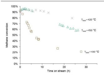
Fig. 5. Time on stream evolution of methane combustion over aged Pd/Al $_2$ O $_3$  catalysts. Feed: 0.7 CH $_4$ , 3.2 % H $_2$ O balance air; GHSV = 100 000 h $^{\text{-1}}$ .  $\square$  = Pd/Al $_2$ O $_3$ -I catalyst (aged 18 h under wet feed at 780 °C);  $\triangle$  = Pd/Al $_2$ O $_3$ -III catalyst (aged 18 h in wet O $_2$  at 780 °C);  $\times$  = Pd/Al $_2$ O $_3$ -IV catalysts (aged 3 days in autoclave at 175 °C).
