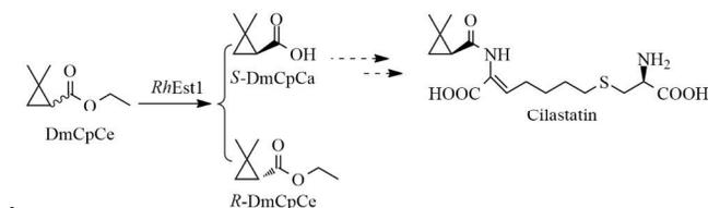
**Scheme 1** Biocatalytic resolution of (±)-DmCpCe for the synthesis of Cilastatin precursor mediated by a novel esterase *RhEst1*.
