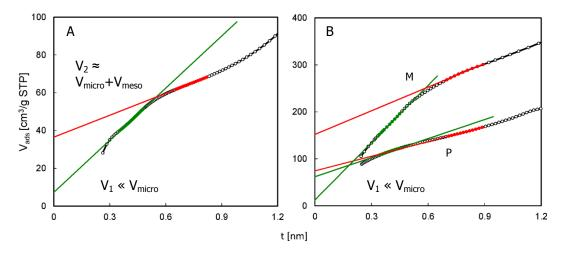
**Figure 11** Application of the t-plot method in adsorption data analysis for hierarchical micromesoporous materials: A) simulated isotherm from Figure 9, B) experimental adsorption data for MCM-56 zeolites: parent (P) and modified by swelling with hexadecyltrimethylammonium-OH/Cl and pillaring with TEOS (M).<sup>219</sup> The corresponding adsorption isotherms are shown in Figure 10A.
