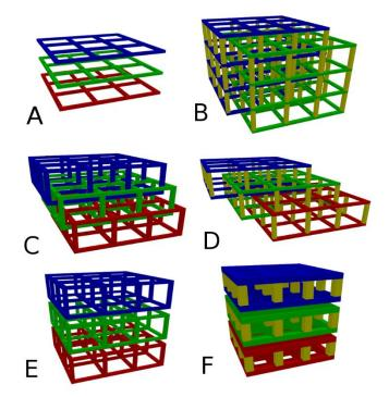
**Figure 4** Schematic representation of 2D MOF structures. A-monolayers; B,C,D-pillared monolayers; C,Ebilayers. B, C, D are interpenetrated structures. F - porosity introduced by pillaring of impermeable layers. Specific examples are discussed in the text.
