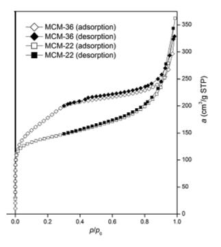
Figure 15 Ar adsorption isotherms observed for MCM-22 and MCM-36 zeolites, adopted from ref. <sup>242</sup>
