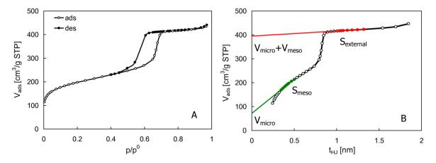
**Figure 10** Illustration of the t-plot method: A) sample isotherm for the model micro-mesoporous material (SBA-15 silica), B) t-plot with the linear segments indicated and extrapolated.
