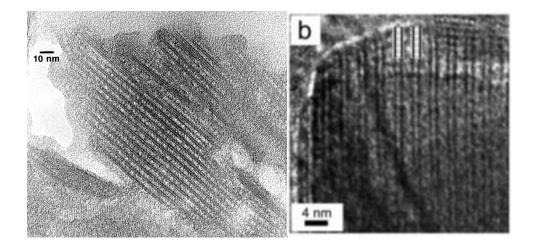
**Figure 8.** HRTEM images of (a) MCM-36 after swelling at 100°C<sup>41</sup>, (b) MCM-22P precursor after swelling at room temperature (Reprinted with permission from J. Am. Chem. Soc. 2008, 130, 1507-1516. Copyright 2008 American Chemical Society). <sup>202</sup>
