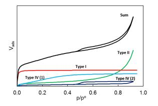
**Figure 9** Sample adsorption isotherm, typical for hierarchical layered micro-mesoporous material constructed as linear combination of type I (Langmuir function), II (BET function) and IV (BET + logistic function) isotherms.
