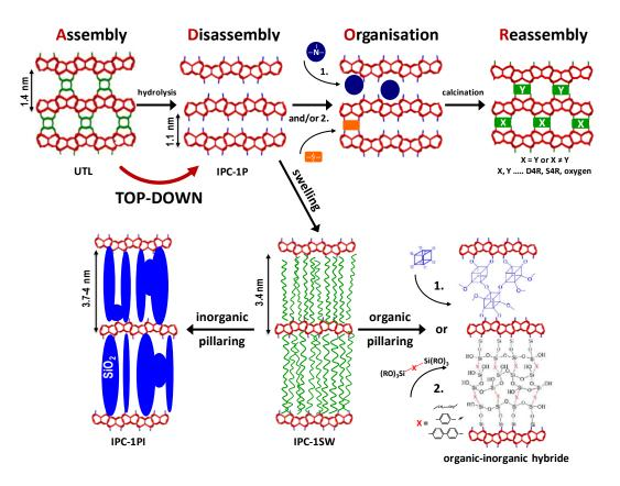
5.3 Top-down preparation of novel layered precursors from zeolites
