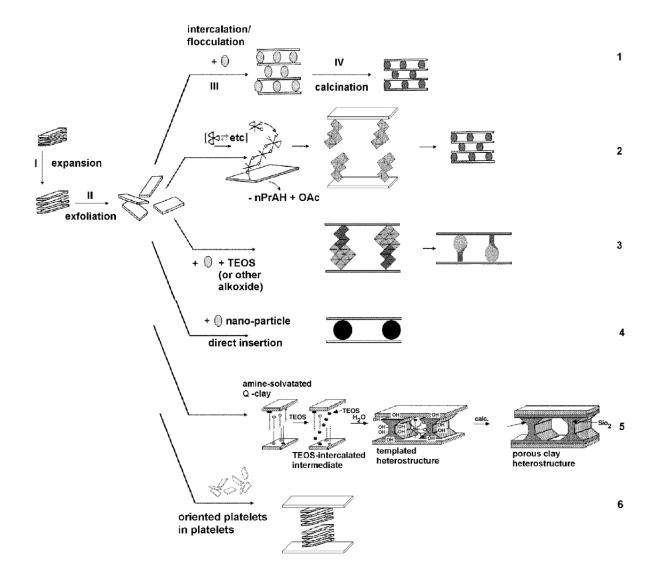
**Figure 5** Different methods for pillaring clays (from top to bottom):<sup>167</sup>1. The traditional Al-Keggin ion route; 2. Surface hydrolysis and polymerization of oxide precursor; 3. Sol-gel intercalation; 4. Intercalation of nano-particles; 5. Porous clay heterostructures; 6. Platelets as pillars (Reprinted from Catalysis Today, Vol. 114, pp. 126-141, A. De Stefanis and A. A. G. Tomlinson, Towards designing pillared clays for catalysis, Copyright 2006, with permission from Elsevier).
