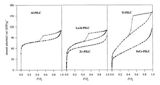
Figure 13 Examples of  $N_2$  adsorption isotherms for montmorillonite pillared with different metal oxides.<sup>234</sup>
