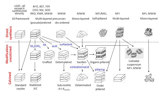
**Figure 2** Principal modifications and structural transformation of layered materials exemplified by 2D zeolites. The representatives for selected layered form are specified with the 3 letter framework code.
