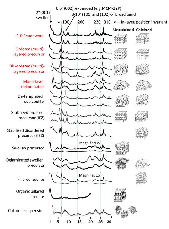
**Figure 7** X-ray diffraction patterns for MWW zeolite materials with different structures. The in-layer (hk0) reflections do not change positions. Interlayer distances are indicated by reflections below 7° 2 $\theta$ , which are in some cases merged with the (100) at 7.1° 2 $\theta$ . The region 8-10° 2 $\theta$  with either resolved or merged (101) and (102) reflections indicates order or disorder, respectively. Materials obtained by direct synthesis are in red.
