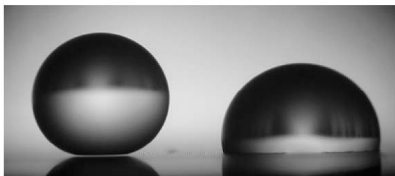
Figure 10. Millimetric water droplets deposited on a superhydrophobic substrate. The light passes below the left droplet indicating the Cassie state, while the right droplet after transition wets the surface in the Wenzel state. Reproduced from Ref. Callies and Quéré 198 .
