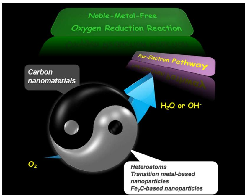
**Fig. 2** Schematic illustration of the high-efficiency carbon nanomaterials-based noble-metal-free oxygen reduction electrocatalysts, which combine the advantages of carbon nanomaterials with large surface area/stable structure and heteroatoms/transition metal-based NPs/ $\text{Fe}_3\text{C}$ -based NPs with high ORR electrocatalytic activity.
