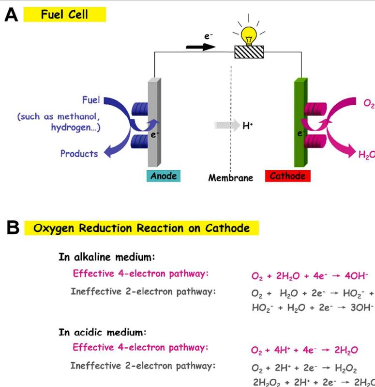
Fig. 1 (A) The typical fuel cells with methanol or H<sub>2</sub> as fuel. (B) ORR pathways in alkaline and acidic media.
