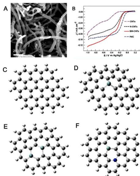
Fig. 8 (A) SEM image of SiN-CNTs. (B) LSV curves of CNTs, N-CNTs, SiN-CNTs and Pt/C in O<sub>2</sub>-saturated 0.1 M KOH solution. The net charge distributions of C, Si and N atoms in pure GN (C), Si-doped GN with one silicon (D) or two silicon atoms (E) and Si, N-co-doped GN (F). (Adapted with permission from Ref<sup>137</sup> Copyright 2015 Royal Chemical Society.)
