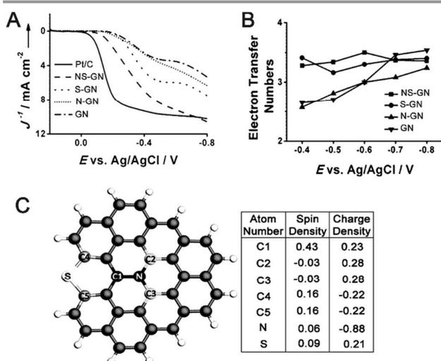
Fig. 17 (A) LSV curves of mesoporous NS-GN, mesoporous S-GN, mesoporous N-GN, mesoporous GN and Pt/C at 1600 rpm. (B) Electron-transfer numbers as a function of the overpotential of different samples. (C) Spin and charge density of GN network dual-doped by N and S. C1 has very high spin density, C2 and C3 have high positive charge density, and C4 and C5 have moderately high positive spin densities. (Adapted with permission from Ref.<sup>127</sup> Copyright 2012 Wiley-VCH Verlag GmbH & Co.)
