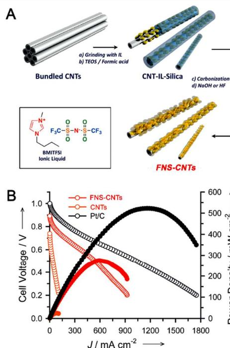
Fig. 9 (A) Synthesis of the FNS-CNTs. (B) The performance of MEAs that employ FNS-CNTs, CNTs, or Pt/C as the cathodes in alkaline fuel cells at 50 °C; open and closed circles correspond to the cell voltages and power densities, respectively. (Adapted with permission from Ref<sup>98</sup> Copyright 2014 Wiley-VCH Verlag GmbH & Co.)
