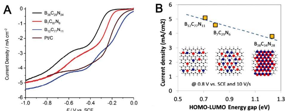
Fig. 12 (A) LSV curves of BN-GN with different compositions and Pt/C catalyst in  $O_2$ -saturated 0.1 M KOH solution. (B) Experiment ORR activities vs. DFT-predicted HOMO-LUMO energy gap for BN-GN. (Adapted with permission from Ref<sup>126</sup> Copyright 2012 Wiley-VCH Verlag GmbH & Co.)
