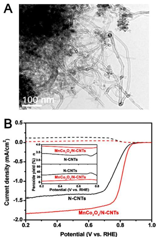
Fig. 20 (A) TEM image of MnCo<sub>2</sub>O<sub>4</sub>/N-CNTs. (B) ORR polarization curves of MnCo<sub>2</sub>O<sub>4</sub>/N-CNTs and N-CNTs. Inset: peroxide yield and electron transfer number per oxygen molecule at various potentials. (Adapted with permission from Ref.<sup>81</sup> Copyright 2014 American Chemical Society.)
