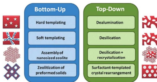
Figure 18: Bottom-up and top-down approaches to hierarchical mesoporous zeolites. (Reproduced with permission from ref. [83], Copyright Wiley-VCH, 2014).
