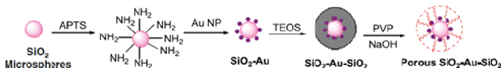
Fig. 14 Schematic representation of the synthesis of a porous SiO 2 -AuNP-SiO 2 core-shell-shell microsphere catalyst. Reprinted with permission from ref. 268 . Copyright 2012 Springer.
