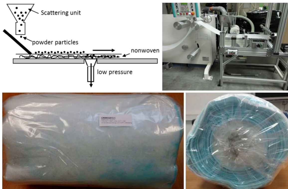
Figure 21 – Continuous and large-scale production process developed by Norafin in the context of NanoMOF project (reference FP7-NMP-2008-LARGE-2). ( Top left ) Principle of the dry loading process and ( top right ) the scattering-suction unit. ( Bottom ) Continuously MOF-particle loaded PET-nonwovens (HKUST-1 <math><63\ \mu\text{m}</math> from Johnson Matthey company; loading capacity: 25 g/m 2 ). [Reprinted from http://cordis.europa.eu/project/rcn/92877_en.html (accessed 02 March 2015).]
