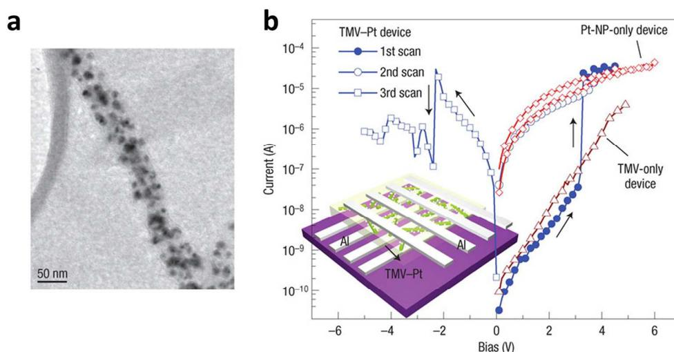
**Figure 24. TMV-based digital memory device. a)** TEM image of TMV with approximately 10 nm-sized Pt nanoparticles uniformly attached. **b)** I-V curves of device created with an active layer derived from the TMV-Pt nanowires (illustrated in inset). The curves demonstrate the
