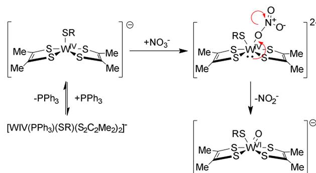
Fig. 14 Mechanism of nitrate reduction to nitrite with Holm's tungsten-centred catalysts as reported in reference 45.
