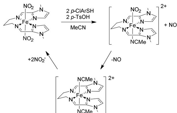
Fig. 7 The structure of complex  $[\text{Fe}(\text{LN}_4^{\text{Im}})(\text{NO}_2)_2]$  and details of its reaction with nitrite in the presence of *p*-chlorobenzenethiol and *p*-toluene sulfonic acid as reported by Harrop.<sup>25</sup>
