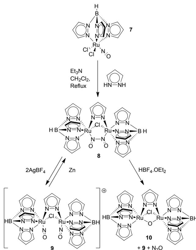
Fig. 11 Onishi's di-ruthenium platform for NO reduction to N<sub>2</sub>O.<sup>33</sup>
