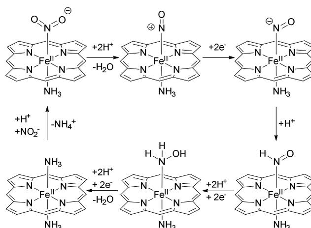
**Fig. 2** Mechanism of nitrite reduction by cytochrome *c* nitrite reductase according to Neese and co-workers.<sup>4</sup>
