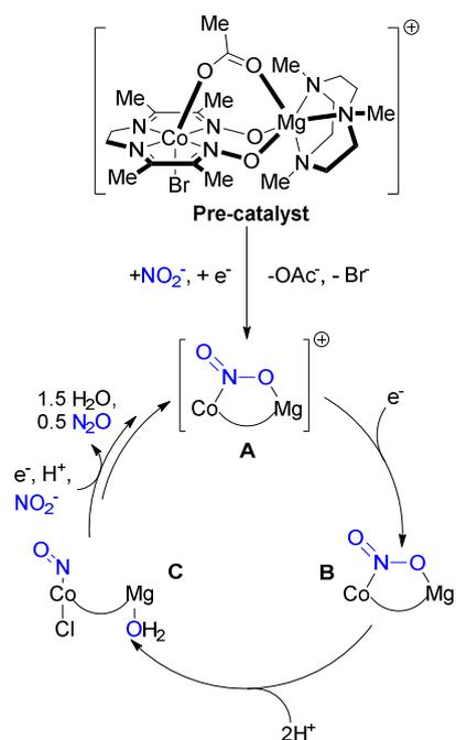
**Fig. 9** The mechanism of  $\text{N}_2\text{O}$  production from nitrite with Uyeda and Peters' bimetallic Co-Mg catalyst.<sup>29</sup>
