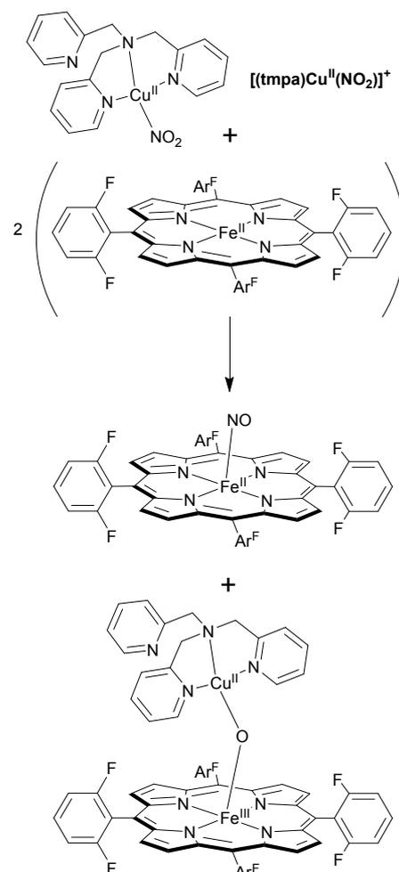
Fig. 10 Nitrite reduction to NO using Karlin's bimetallic haem-Cu tripod system.<sup>30</sup>
