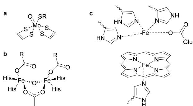
Fig. 4 a) Simplified active site structure of the dissimilatory nitrate reductases, showing the primary coordination environment around the Mo centre. SR is typically cysteine. Alternatively, this ligand could be present as -OR in the form of serine. b) Active site structure of flavodiiron nitric oxide reductase, FNOR. The R-groups on FNOR are either aspartate or glutamate. His = histidine. c) Simplified active site structure of nitric oxide reductase. Glu = glutamate.
