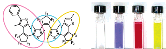
Fig. 19 Colour changes in 61 when closing one of the three DTE units. The black coc (not shown) form can be obtained also. Adapted with permission from Ref. 164, Copyright 2005 American Chemical Society.
