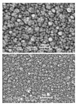
**Fig. 9** SEM images of a nano-structured Ni(II)-curcumin-modified carbon electrode at two different magnifications (50.000x and 60.000x). Reproduced from ref. 48. Copyright 2008 Elsevier B. V.
