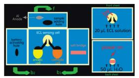
Fig. 21 Schematic illustration of the working principle of the self-powered 3D microfluidic ECL biosensing device. f: front sheet; b1: the sheet folded to the back first; b2: the back sheet. Reprinted with permission from ref. 106.
