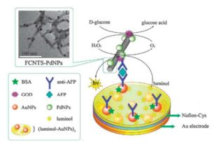
Fig. 22 Schematic diagram of the ECL-based sandwich-type immunosensor for 30 detection of  $\alpha$ -1-fetoprotein. Reprinted with permission from ref. 115.
