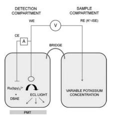
Fig. 29 Schematic representation of the electrochemical device with two 15 separated sections (sample and detection) used to indicate the ECL readout conception for potentiometric sensors. Reprinted with permission from ref. 164.
