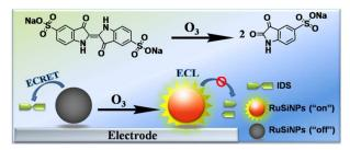
40 Fig.17 Scheme for the principle of ECL resonance energy transfer determination of ozone combined with RuSiNPs and indigo carmine. Reprinted with permission from ref. 98.
