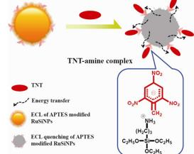
Fig.18 Schematic illustration of ECL turn-off detection of TNT by using APTES-modified RuSiNPs based on an ECL resonance energy transfer mechanism. Reprinted with permission from ref. 99.
