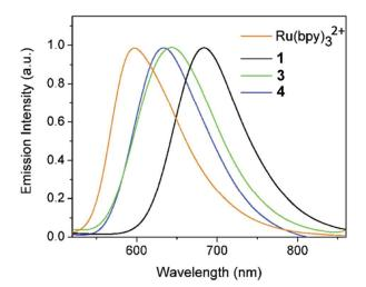
25 Fig. 3 Normalized photoluminescence spectra obtained from thin solid films of compounds 1, 3, 4, and Ru(bpy)<sub>3</sub>·2PF<sub>6</sub> with excitation wavelength at 450 nm. Reprinted with permission from ref. 14.
