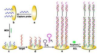
Fig. 23 Schematic representation of the preparation of the hybridization chain reaction-based ECL DNA sensor. Reprinted with permission from ref. 119.
