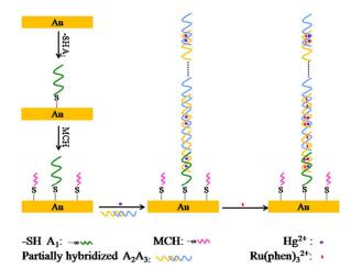
Fig. 25 Schematic diagram of the label-free supersandwich sensing platform  $_{60}$  for ECL detection of Hg<sup>2+</sup>. (yellow curve, A2; blue curve, A3). Reprinted with permission from ref. 132.
