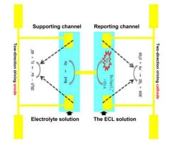
Fig. 26 Schematic illustration of the fundamental principle of the dual-channel bipolar ECL sensor. Reprinted with permission from ref. 155.
