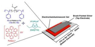
20 Fig. 31 Schematic representation of an ECL device based on an ECL emissive gel layer consisted of Ru(bpy)<sub>3</sub>Cl<sub>2</sub>/PS-b-PMMA-b-PS/[EMI][TFSI] in the weight ratio 1:4:16 and a brush-painted top Ag electrode. Reprinted with permission from ref. 184.
