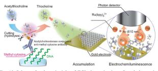
Fig. 19 Scheme for the principle of ECL determination of methyl-cytosine. Reprinted with permission from ref. 102.
