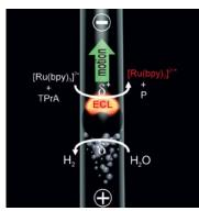
Fig. 27 Asymmetric light-emitting electrochemical swimmer. Reprinted with permission from ref. 157.
