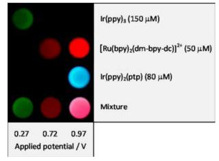
Fig. 9 Pictures of the ECL at the glassy carbon electrode surface at different <sup>75</sup> applied potentials. Reprinted with permission from ref. 46.
