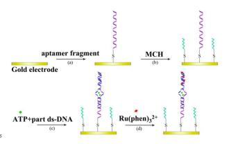
Fig. 24 Schematic representation of the label-free ECL-based aptasensor for detection of ATP. Reprinted with permission from ref. 131.
