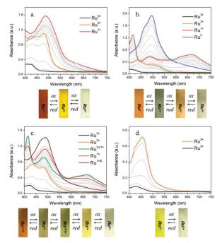
Fig. 30 Spectroelectrochemistry data and the corresponding photos of the polymeric films of 1 (a), 2 (b), 1 and 2 mixture in 1:1 molar ratio (c), and 3 (d) <sup>85</sup> at all the unequivocally stable redox states in 0.1 M tetrabutylammonium hexafluorophosphate acetonitrile solutions. Structure of the acrylate-containing Ru(bpy)<sub>3</sub><sup>2+</sup>-based coordination complexes 1, 2, and 3 were shown in fig. 2. Reprinted with permission from ref. 14.
