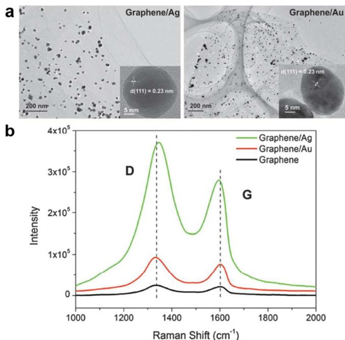
**Figure 2** Raman signal enhancement of graphene using SERS. (a) TEM images of graphene/Au and graphene/Ag nanocomposites. The insets are the corresponding HRTEM images. (b) Raman spectra of graphene, graphene/Au and graphene/Ag nanocomposites in their aqueous dispersions. Reproduced from ref 33 with permission from the PCCP Owner Societies.
