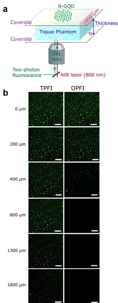
**Figure 8** Two-photon fluorescence deep tissue imaging. (a) Schematic of the measurement setup. (b) Penetration depth of N-GQDs for TPF (two-photon fluorescence imaging) and OPFI (one-photon fluorescence imaging) in tissue phantom. Reprinted with permission from ref 109, copyright 2013 American Chemical Society.
