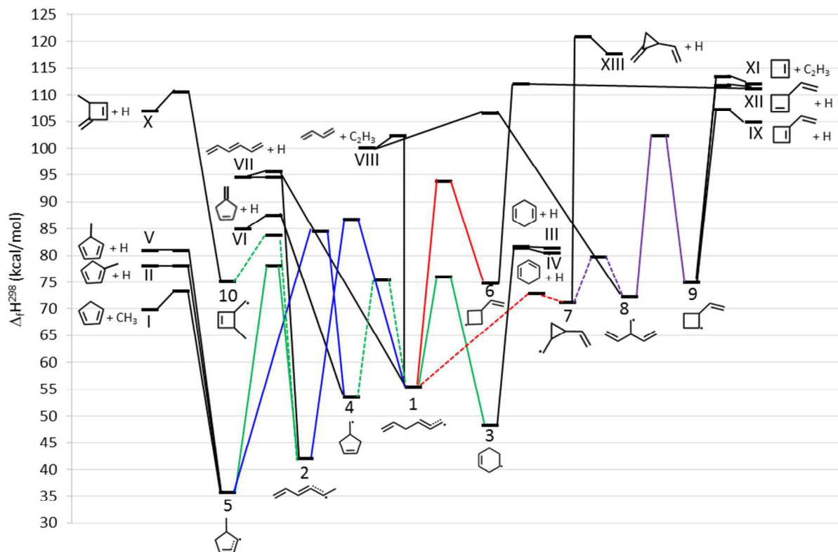
Figure 7: Simplified C_6H_9 potential energy surface calculated at the CBS-QB3 level of theory, showing the enthalpies in kcal/mol at 298K. The cycloaddition reactions are shown by the blue lines (scheme 3), red lines (scheme 1), and the purple lines. For these reactions the dashed lines correspond to the exo-pathway and the solid lines to the endo-pathway. The blue lines correspond to H-atom shift reactions and the black lines to \beta -scission reactions.
