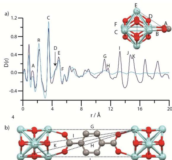
**Figure 6.** (a) PDF data for UiO-66 (dark blue) and a<sub>m</sub>UiO-66 (light blue). A-F labels of peaks below 8 Å correspond to the indicated correlations in the Zr<sub>6</sub>O<sub>4</sub>(OH)<sub>4</sub> cluster (Inset). (b) Two Zr<sub>6</sub>O<sub>4</sub>(OH)<sub>4</sub> units linked by a bdc ligand, and some of the significant distances corresponding to the longer *r* features (G-K) in (a). Zr – light blue, O – red, C – gray, H – omitted.
