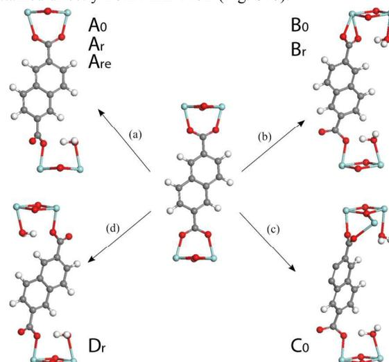
**Figure 5.** Formation of different types of defective structures upon direct binding of water on a Zr-center. The names of the defective models derived from each pathway are included for clarity. Zr – light blue, O – red, C – gray, H – white.
