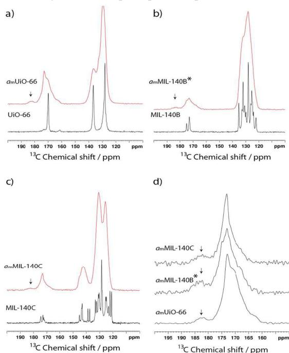
**Figure 3.**  $^{13}\text{C}$  MAS NMR spectra of crystalline (black) and amorphous (red) samples of (a) **UiO-66**, (b) **MIL-140B** and (c) **MIL-140C**. (d) Magnified view of the 150-200 ppm region of the amorphous samples. Acquisition parameter details are given in the SI.
