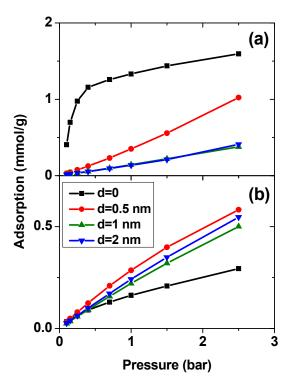
Figure 6. Selectivity of SO<sub>2</sub> over N<sub>2</sub>, computed by the GCMC simulations, in a binary mixture (1:99) on double-walled carbon nanotube arrays, with inner tube diameter 2R=3 nm and intertube distance d=0-2 nm. T=303 K.
