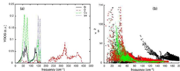
**Figure 3** (a) Total vibrational DOS of BiOCuSe projected on each element. (b) Mode-resolved Grüneisen parameter versus mode frequency for BiOCuQ with Q = S (black), Se (red), Te (green). Phonon frequencies were computed using the experimentally determined structures at 293K.
