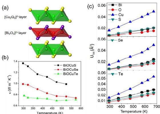
**Figure 1.** (a) Polyhedral view of the crystal structure of BiOCuQ; (b) total thermal conductivity as a function of temperature; (c) ADPs for BiOCuQ as a function of temperature.
