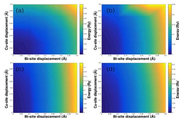
**Figure 4.** Total energy response to atomic displacements of Bi and Cu in BiCuOS. The displacements were done along inequivalent tetragonal directions: (a) Bi along x and Cu along x, (b) Bi along z and Cu along x, (c) Bi along +z and Cu along +z, and (d) Bi along -z and Cu along +z.
