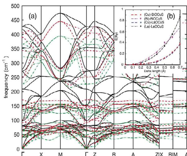
**Figure 2.** (a) Phonon dispersion curves for BiOCuQ. Key: black solid line: BiOCuS; red dashed line: BiOCuSe; green dash-dot line: BiOCuTe. The inset (b) shows the total energy response to the compression of Cu-S, La-O, and Bi-O bonds in BiOCuS and LaOCuS.
