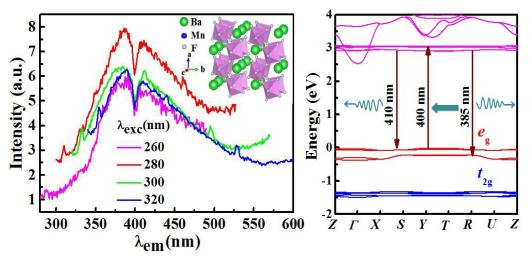
Strong room-temperature blue-violet photoluminescence in  $BaMnF_4$  is derived from Mott gap mediated d-d orbital transitions, and the unusual abrupt drop of luminescence intensity at wavelength of 400 nm was caused by photon self-absorption effect.
