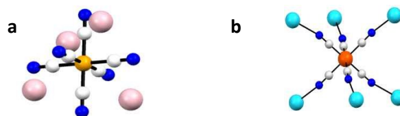
Fig. 1: a) K_4Fe(CN)_6 cluster. b) Fe-(\mu CN)_6-Th_6-\delta_x cluster. Iron - orange, carbon - white, nitrogen - blue, potassium - pink and thorium - light blue (partial charges are not shown).
