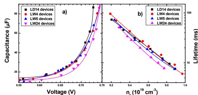
**Fig. 7** Transient photovoltage decay and charge extraction measurements of LD14, LW4, LW5, and LW24 based DSSC devices. a) Comparisons of chemical capacitance at a certain open-circuit photovoltage; b) Comparisons of electron lifetime at a given electron density.
