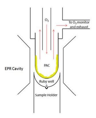
Figure 2. Experimental flow system schematic. A Teflon cylindrical rod, labelled 'Sample Holder,' was used to ensure the EPR tube was placed in the same spot in the EPR cavity between experiments. This
