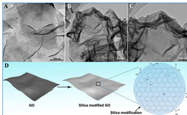
**Fig. 4.** TEM images of GO (A), low- (B) and high-magnification (C) TEM images of silica modified GO. Schematic illustration for the silica modification process (D).
