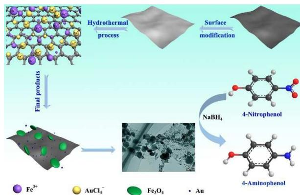
**Scheme 1.** Schematic illustration of the formation process of  $\text{rGO}/\text{Fe}_3\text{O}_4/\text{Au}$  composite.
