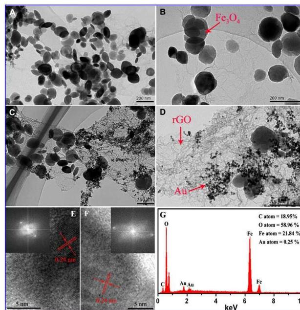
**Fig. 5.** Low- (A) and high-magnification (B) TEM images of rGO/Fe<sub>3</sub>O<sub>4</sub> composite, low- (C) and high-magnification (D) TEM image of rGO/Fe<sub>3</sub>O<sub>4</sub>/Au composite, HRTEM image of rGO/Fe<sub>3</sub>O<sub>4</sub>/Au composite (E, F) and EDS (G). The insets in (E) and (F) are corresponding FFT patterns.
