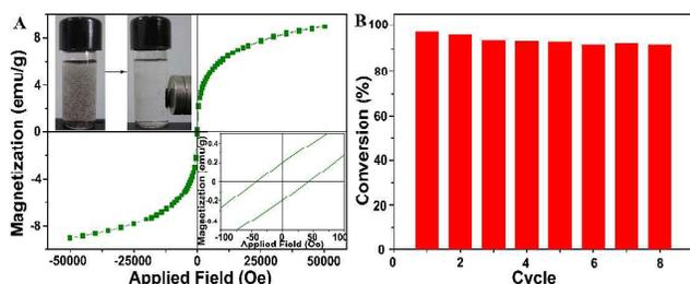
**Fig. 9.** Magnetization curve of rGO/Fe<sub>3</sub>O<sub>4</sub>/Au at room temperature (A), The inset shows the photographs of the magnetic separation. The reusability of rGO/Fe<sub>3</sub>O<sub>4</sub>/Au catalyst (B).
