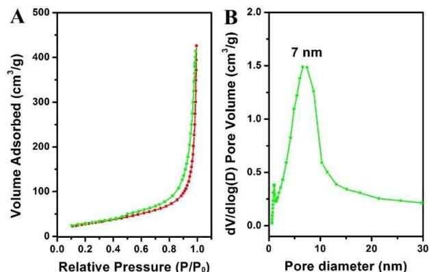
**Fig. 6.**  $\text{N}_2$  adsorption-desorption isotherms (A) and particle size distribution (B) of  $\text{rGO}/\text{Fe}_3\text{O}_4/\text{Au}$  composite.
