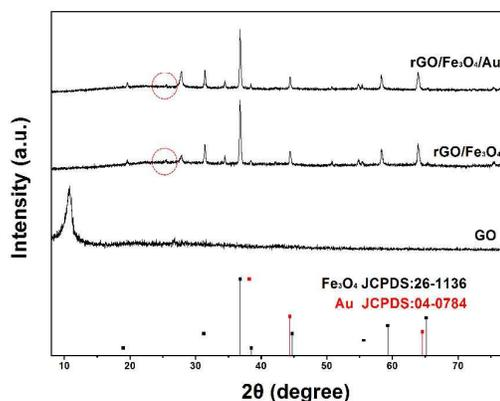
Fig. 1. XRD patterns of the pristine GO, rGO/Fe<sub>3</sub>O<sub>4</sub> and the rGO/Fe<sub>3</sub>O<sub>4</sub>/Au composite.
