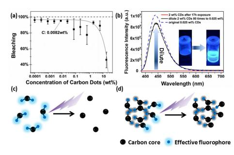
Fig. 7 (a) Percentage of fluorescence bleaching as a function of CD concentration. (b) After dilution, the fluorescence intensity of the exposed concentrated CD suspension is almost recovered to the value of the as-prepared diluted sample. (c) Schematic diagram to explain fluorescence photobleaching of low concentrated CD suspensions. (d) Schematic diagram to explain photobleaching of highly concentrated CD suspensions.
