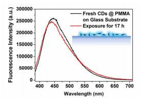
Fig. 12 Luminescence spectra of CDs@PMMA on glass substrate before and after exposure to UV light.
