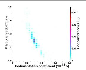
Fig. 9 Pseudo-3D plot of the CDs after UV-exposure. A slight increase in polydispersity is found for the treated sample. The sedimentation coefficient is shown for water at standard conditions (20°C).
