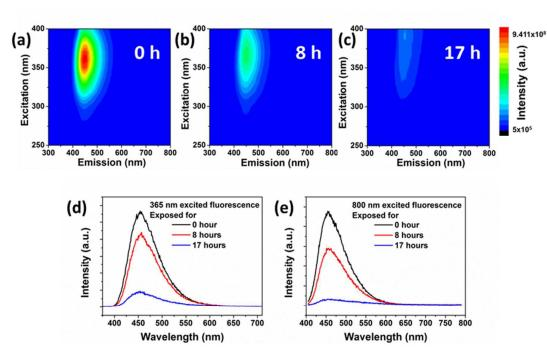
Fig. 6 3D-luminescence plots of CDs after (a) 0, (b) 8 and (c) 17 hours of UV-exposure in aqueous solution at room temperature. Intensity rises from blue to green and to red. The luminescence spectra of CDs in aqueous solutions upon (d) 365 and (e) 800 nm excitation at room temperature, respectively.
