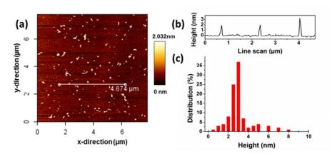
Fig. 1 (a) AFM image of carbon dots (CDs) on a mica substrate,  $8 \times 8 \mu m$ . (b) Measured height profile along the white line in (a). (c) Height distribution from analysis of the AFM images.
