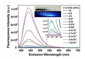
Fig. 4 Self-quenching of the CD fluorescence. The insets show the photos of different concentrated CD suspensions under sun light (above) and UV light (below).
