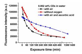
Fig. 8 Kinetics of UV-induced fluorescence photobleaching of a suspension of 0.002 wt.% CDs in water in the absence of oxygen and in the presence of it and in the presence of ascorbic acid.
