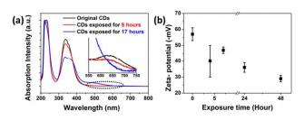
Fig. 11 (a) Absorption spectra of CDs recorded after different UV exposure time, the illustration is an enlarged plot of the dotted line area. (b) Zeta-potential of the CD samples as a function of UV exposure time.
