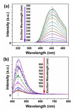
Fig. 3 The excitation-wavelength independent fluorescence spectra of CDs in (a) normal fluorescence and (b) up-conversion fluorescence.
