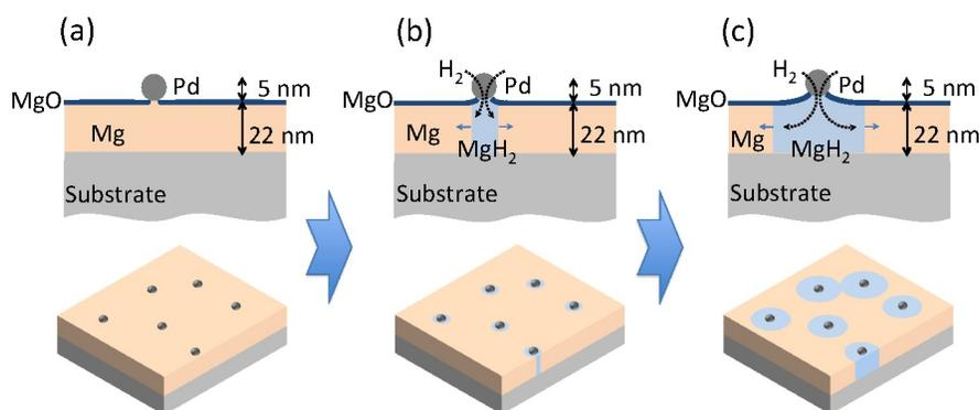
**Fig. 1** A schematic diagram of the novel Pd nanoparticle nano-portal structure and the predicted hydrogenation mechanism. The upper part of the figure is the structure in cross section and the lower part is the structure visualized in three dimensions. (a) The structure of the as-grown sample. (b) The nucleation of  $\text{MgH}_2$ . (c) The growth process of the nucleated  $\text{MgH}_2$ .
