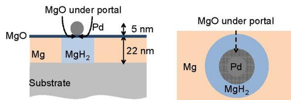
**Fig. 5** The portal pinches off under the Pd nanoparticle. On the right is an exaggerated top view showing a decreased area of portal and hence a lowered H flux.
