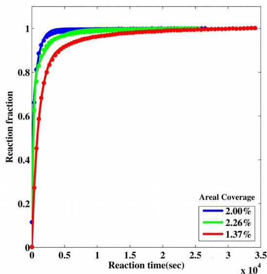
**Fig. 8** Model fits to observed behavior incorporating portal pinch-off and an additional leak flux through the MgO, for the low coverage samples. The solid lines are fits to the data.
