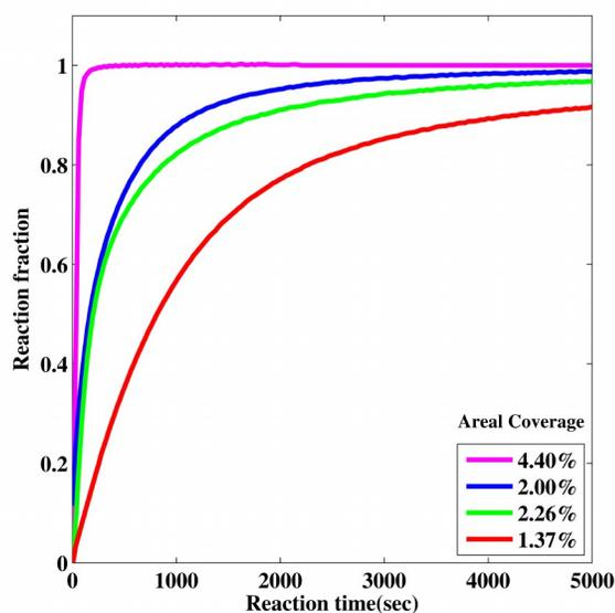
**Fig. 6** Effect of Pd nanoparticle coverage on hydrogenation reaction rate. Hydrogenation reaction curves of samples with different Pd nanoparticle coverage (~1.7%~6.3%) grown on epitaxial Mg films.
