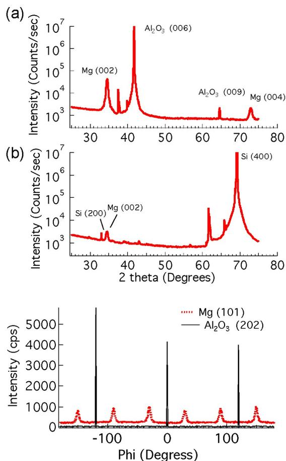
**Fig. 2** X-ray diffraction  $\theta$ - $2\theta$  scans of as deposited 22 nm Mg with Pd nanoparticles. (a) Samples that were grown on a sapphire substrate. (b) Samples that were grown on a silicon substrate. The unlabeled peaks are all from substrates. (c) X-ray diffraction phi scans of an epitaxial Mg film. The sample was grown on an (0001)  $\text{Al}_2\text{O}_3$  substrate with Pd nanoparticles deposited on the surface.
