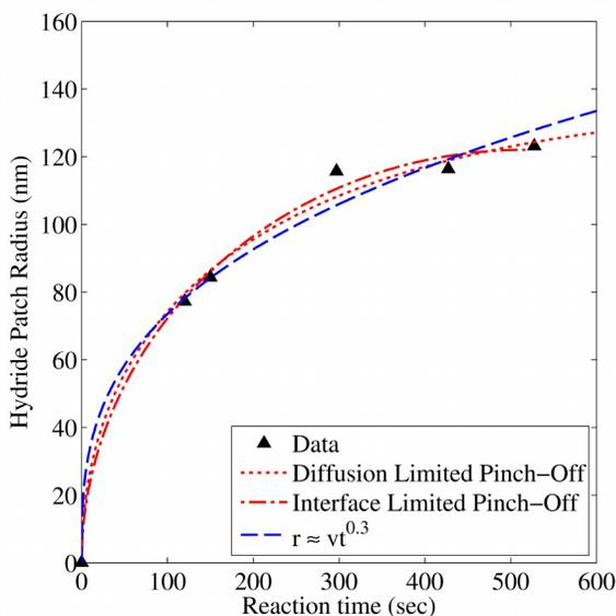
**Fig. 4** Model fits to explain time dependence of the measured average radii of the hydride patches grown in epitaxial Mg samples. The agreement is seen to be much better for the models incorporating the oxidation under the portals
