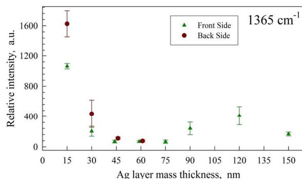
Figure 6. Intensity of the  $1365 \text{ cm}^{-1}$  band in SERS spectra of CuTMPyP4 adsorbed on the silvered surface of AAO as a function of the silver film thickness. Data obtained at front- and back-side geometry of excitation are depicted by triangles and circles, respectively. The symbols for samples of  $h=45 \text{ nm}$  and  $h=60 \text{ nm}$  have been horizontally offset for clarity.
