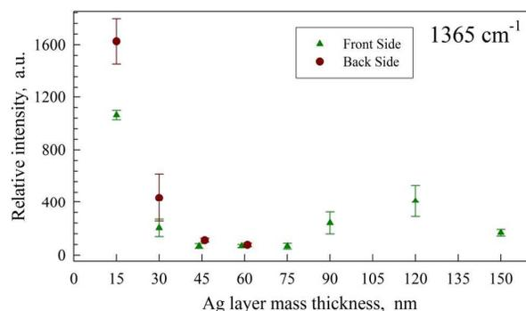
Figure 6. Intensity of the  $1365 \text{ cm}^{-1}$  band in SERS spectra of CuTMPyP4 adsorbed on the silvered surface of AAO as a function of the silver film thickness. Data obtained at front- and back-side geometry of excitation are depicted by triangles and circles, respectively. The symbols for samples of  $h=45 \text{ nm}$  and  $h=60 \text{ nm}$  have been horizontally offset for clarity.
