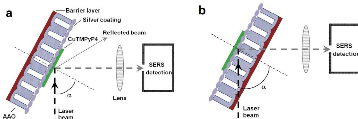
Figure 4. The excitation-detection geometries of SERS measurements: (a) front-side excitation; (b) back-side excitation. Incident angle  $\alpha = 57^\circ$ .
