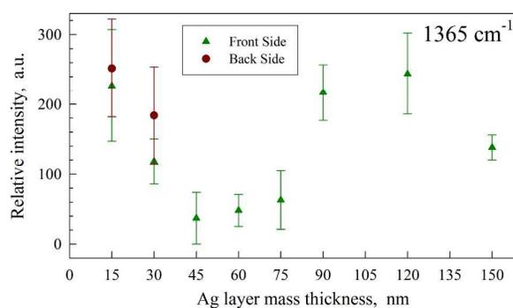
Figure 7. Intensity of the  $1365 \text{ cm}^{-1}$  band in SERS spectra of CuTMPyP4 deposited on the silvered surface of AAO by dropping from  $10 \mu\text{l}$  of  $10^{-6}$  M solution as a function of the silver film thickness. Data obtained at front- and back-side geometry of excitation are depicted by triangles and circles, respectively.
