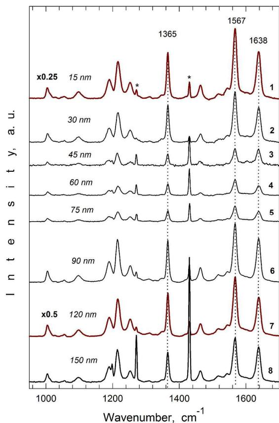
Figure 5. SERS spectra of CuTMPyP4 adsorbed from the  $10^{-6}$  M solution on the surface of Ag/AAO with silver film thickness of 15 (1), 30 (2), 45 (3), 60 (4), 75 (5), 90 (6), 120 (7) and 150 nm (8). Prominent plasma lines of He-Cd laser are marked with asterisks (\*).
