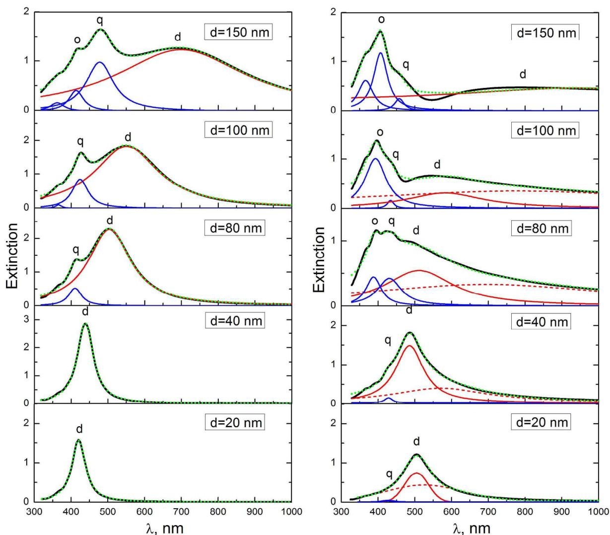
Figure 3. Calculated extinction spectra and tentative assignment of SPR modes for sparse colloids of Ag NPs (left panel) and close-packed monolayers (right panel) of Ag nanoparticles of different diameters  $d$ . d – dipole mode; q – quadrupole mode; o – octupole mode.
