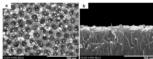
Figure 1. SEM images of Ag/AAO sample with a thickness of silver film ca 60 nm: (a) the top view and (b) the cross-sectional view.
