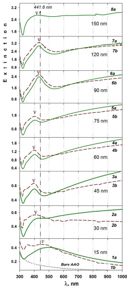
Figure 2. Extinction spectra of Ag/AAO samples with different Ag film thickness: 1a,b - 15 nm; 2 a,b - 30 nm; 3 a,b - 45 nm; 4 a,b - 60 nm; 5 a,b - 75 nm; 6 a,b - 90 nm; 7 a,b - 120 nm; 8a - 150 nm. Spectra 1a – 8a were measured at normal incidence, spectra 1b – 7b at the angle  $57^\circ$ . Dash-dot-dot arrow indicates position of excitation wavelength 441.6 nm.
