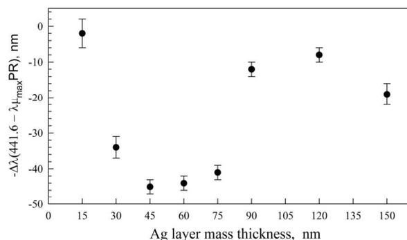
Figure 8. Difference between position of extinction maximum and excitation wavelength as a function of the silver film thickness. Peak maxima were determined for spectra measured at incident angle  $\alpha = 57^\circ$ .
