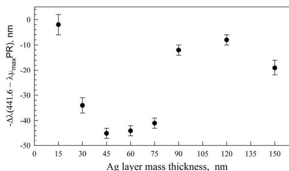
Figure 8. Difference between position of extinction maximum and excitation wavelength as a function of the silver film thickness. Peak maxima were determined for spectra measured at incident angle  $\alpha = 57^\circ$ .
