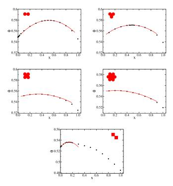
**Fig. 5** (Color online) Saturated packing fraction dependence on parameter x for trimers, tetramers, hexamers and square dimers. Dots represents data from numerical simulations. Error bars are smaller than dots sizes. Solid red lines are quadratic fits near maxima of  $\theta_{\rm max}$ . Data for dimers were taken from  $^{22}$ . The fits are:
