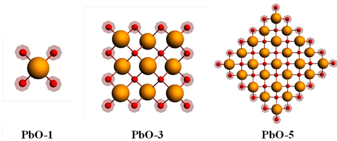
**Figure 3.** 1<sup>st</sup>, 3<sup>rd</sup> and 5<sup>th</sup> co-ordination shell geometries of  $\alpha$ -PbO. The terminal oxygen atoms are shown in red circles. The corresponding  $\beta$ -PbO clusters have the same bonding network with differences in bond lengths and angles.
