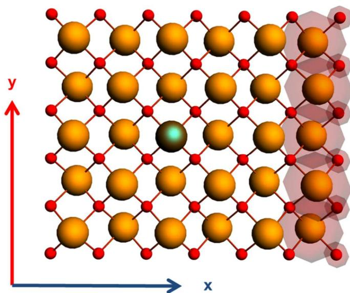
**Figure 4.** Distorted 5<sup>th</sup> co-ordination shell cluster of  $\alpha$ -PbO. The added co-ordination in x-direction is shown in red circles whereas the central  $^{207}\text{Pb}$  nuclei is highlighted.
