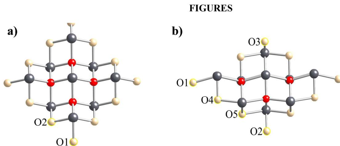
**Figure 1.** Different terminal oxygen sites according to bond valence model in a)  $\alpha$ -PbO and b)  $\beta$ -PbO.
