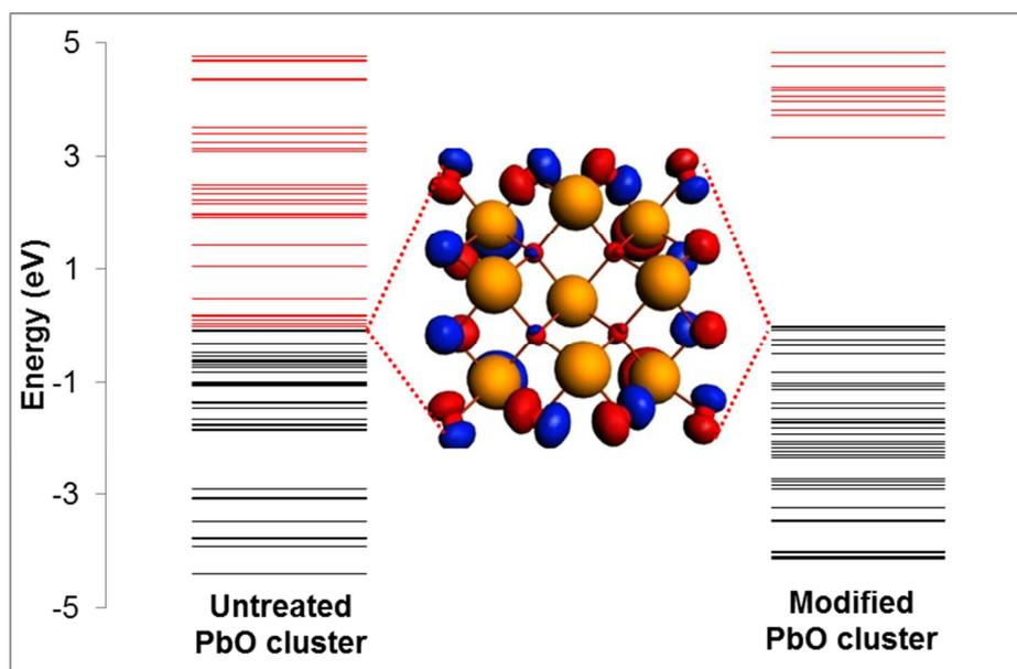
**Figure 2.** Energy levels for the 3<sup>rd</sup> co-ordination cluster of  $\alpha$ -PbO. The occupied levels are shown in black whereas unoccupied levels are shown in red. These qualitative calculations carried out with BP86 functionals and the ZORA spin-orbit Hamiltonian.
