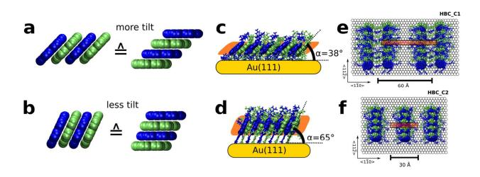
**Fig. 2 Effect of tilt angle on resulting lateral shift and packing density:** (a-b), Two different perspective views of HBC-discs showing the effect of tilt angle on the resulting lateral shift. (c), Side view of proposed structural model of mono-thiolate HBC (HBC\_C1) and top view shown in (e). Side view of di-thiolate HBC SAM (HBC\_C2) depicted in (d) and corresponding structural model in (f).
