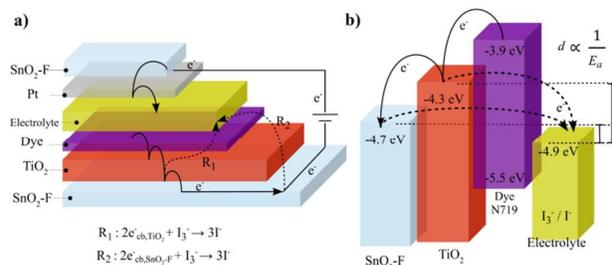
**Fig. 1** a) Schematic representation of the working principles at a dye sensitized solar cell; and b) diagram of energy levels of each functional layer in the DSC. The full arrows represent electron pathways through the device; the dashed arrows represent the main loss reaction mechanisms due to recombination through TiO<sub>2</sub> or SnO<sub>2</sub>-F interfaces ( $R_1$  and  $R_2$ , respectively). The actual energy levels may change upon assembling.
