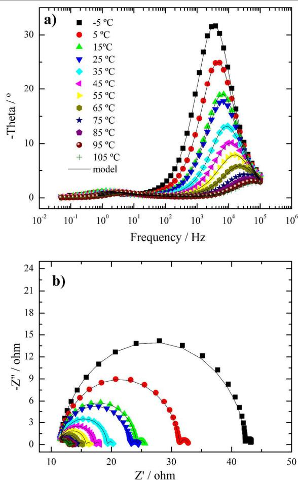
Fig. 7 Platinum half-cell Bode (a) and Nyquist (b) plots obtained in dark conditions at 0 V in the temperature range -5 to 105 °C.
