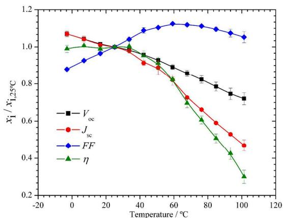
Fig. 6 Performance parameters normalized to the corresponding values 25 °C values ( $V_{OC,25°C} = 0.777$  V ;  $J_{SC,25°C} = 9.5$  mA·cm<sup>-2</sup>), as a function of the operating temperature. Lines were added for readability.
