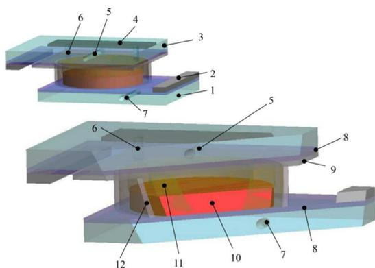
**Fig. 2** Schematics of the manufactured DSC device (not in scale): 1 – Photoelectrode glass; 2 – electrical contact; 3 – counter-electrode glass; 4 – filling hole cover; 5 – drilled hole for temperature measurement,  $T_2$ ; 6 – filling hole; 7 – drilled hole for temperature measurement,  $T_1$ ; 8 – TCO; 9 – platinum catalyst; 10 –  $\text{TiO}_2$  with adsorbed sensitizer; 11 – electrolyte; 12 – glass frit sealing.
