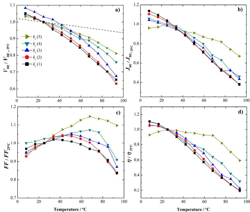
**Fig. 12** *I-V* performance parameters relative to 25 °C values of five different batches of DSCs differing in the recombination reaction constant  $k_{r(\eta)}$ . The black dashed line in a) corresponds to the theoretical  $V_{OC}$  vs. temperature trend expected for a cell with no recombination (calculated from the Butler-Volmer equation<sup>64</sup>). Lines were added for readability.
