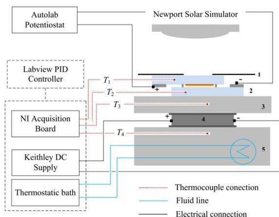
**Fig. 3** Experimental setup used for temperature control of an under illumination DSC between  $-5\text{ }^{\circ}\text{C}$  and  $105\text{ }^{\circ}\text{C}$ . 1- thermal insulator black mask; 2- DSC; 3- aluminum slab; 4- peltier device; 5- aluminum slab with drilled thermal fluid circuit.
