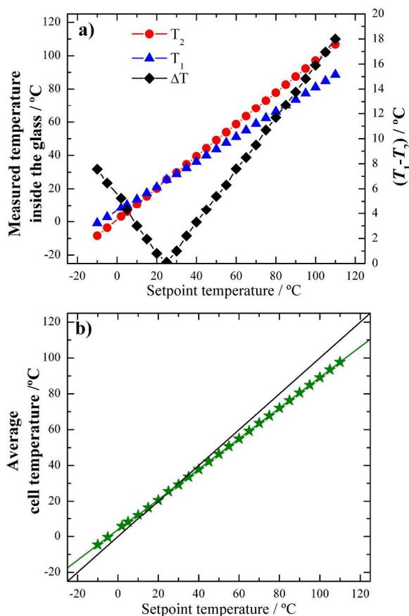
**Fig. 4** Temperature values from: a)  $T_1$  (photoelectrode),  $T_2$  (counter electrode), calculated temperature difference between electrodes; and b) average cell temperature versus set point temperature.
