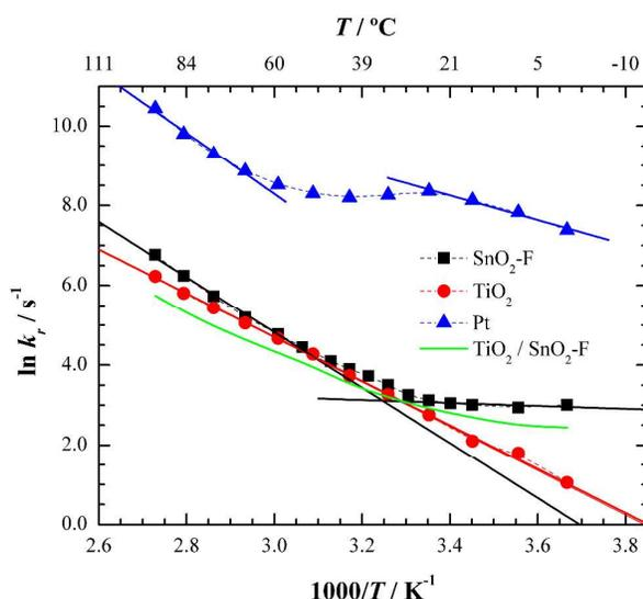
Fig. 14. Arrhenius plot of recombination reaction (reduction of triiodide) for three types of half-cells: SnO<sub>2</sub>-F, TiO<sub>2</sub> blocking layer and Pt. The green curve represents the average between the TiO<sub>2</sub> and SnO<sub>2</sub>-F curves.
