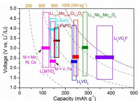
Fig. 1 Typical operating voltage/capacity range/energy density plots for various reported DRS (space group *Fm-3m*) cathode materials for Li-ion batteries.<sup>18–24</sup> The bars indicate the average voltages.  $\text{LiFePO}_4$  and  $\text{LiCoO}_2$  are also shown for comparison.
