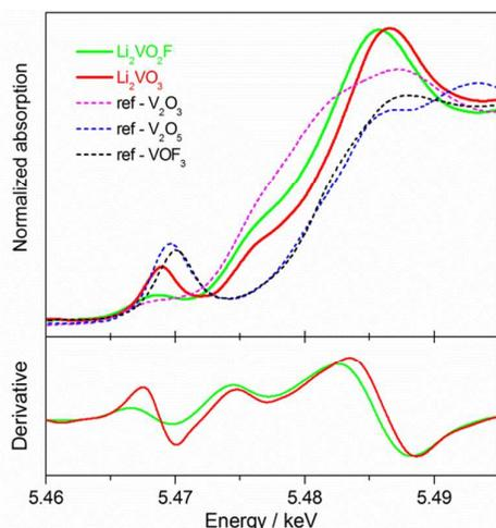
Fig. 4 V K-edge XANES spectra and the derivative plots for  $\text{Li}_2\text{VO}_2\text{F}$  and  $\text{Li}_2\text{VO}_3$ .
