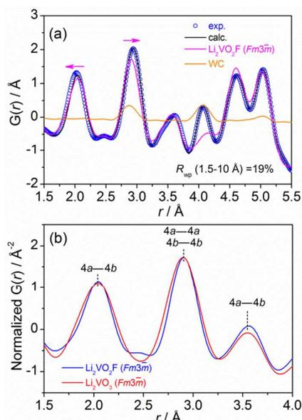
**Fig. 3** (a) Experimental and calculated (using Rietveld average structure model) atomic PDF profile for  $\text{Li}_2\text{VO}_2\text{F}$ ,  $U_{\text{iso}}(\text{\AA}^2)$  parameters for Li, V, O and F are 0.0024, 0.0122, 0.0128 and 0.1721, respectively. (b) Modelled PDF profiles for two  $Fm\text{-}3m$  phases with oxo and oxofluoro anion ligands in the  $r$ -range of 1.5–4  $\text{\AA}$ .
