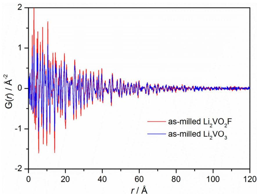
**Fig. S2** Experimental atomic PDF profiles,  $G(r)$ , for the as-milled  $\text{Li}_2\text{VO}_2\text{F}$  and  $\text{Li}_2\text{VO}_3$ . The primary crystallite sizes for both materials are about 10 nm.
