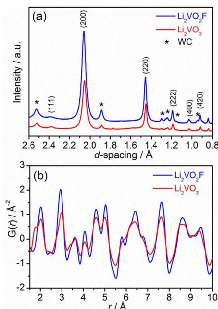
Fig. 2 (a) Synchrotron XRD patterns ( $\lambda = 0.41343$   $\text{\AA}$ ), and (b) atomic PDF profiles in the  $r$ -range from 1.5 to 10  $\text{\AA}$  for  $\text{Li}_2\text{VO}_2\text{F}$  and  $\text{Li}_2\text{VO}_3$ .
