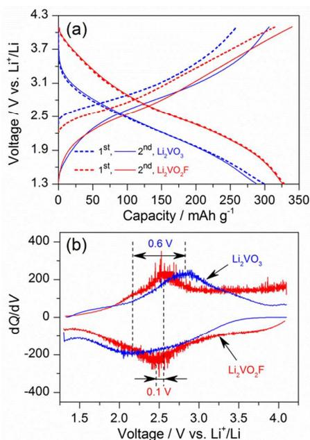
Fig. 5 (a) Voltage profiles for  $\text{Li}_2\text{VO}_3$  and  $\text{Li}_2\text{VO}_2\text{F}$  measured between  $1.3$  and  $4.1 \text{ V}$ . (b)  $dQ/dV$  plots from the second cycles.
