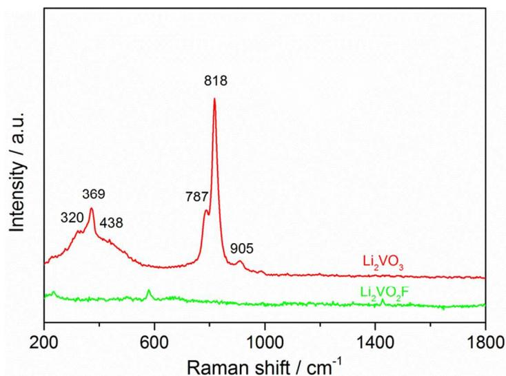
**Fig. S4** Raman spectra of the as-milled Li<sub>2</sub>VO<sub>2</sub>F and Li<sub>2</sub>VO<sub>3</sub>.
