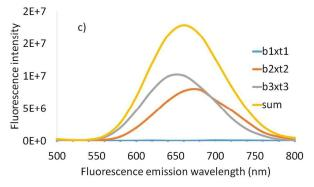
Figure 4. Decay associated spectra of BSA-AuNC at (a) pH 1; (b) pH 7; and (c) pH12. Three exponential fitting gave (a) t1 =220 ns, t2=1940 ns, t3=4460 ns; (b) t1=360 ns, t2=2000 ns, t3=4730 ns; (c) t1=190 ns, t2=1170 ns, t3=2400 ns.
